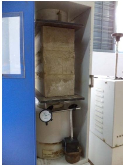
Fig 3.8(b) Load Test on prism in progress
