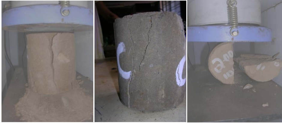
Fig 4.28 Failure pattern in Compression and Tension (No Fibre)
