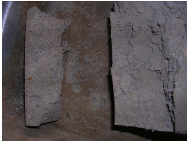
Fig 4.31 Slipping of Bottle fibre from Soil Cement matrix
