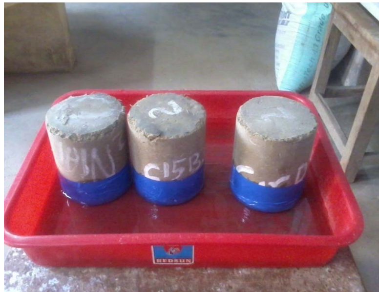
Fig 3.9 Sorptivity test in progress
