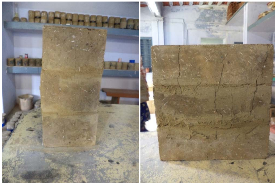
Fig 4.33 Failure of masonry prism (blocks with Kit fibre)
