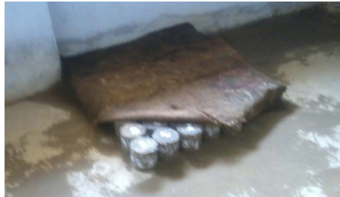
Fig 3.5 Curing of Cylindrical specimens in progress
