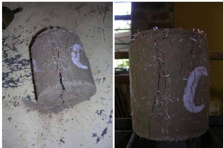
Fig 4.29 Failure pattern in Compression (samples with Kit fibre)
