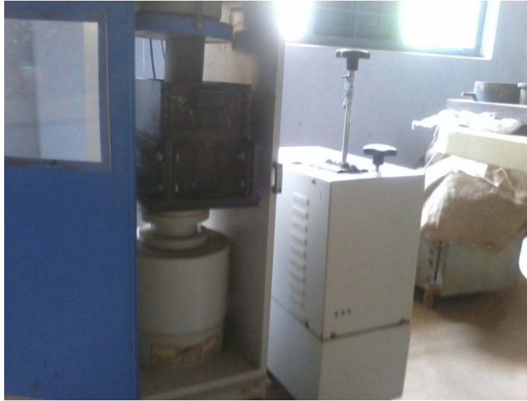
Fig 3.6(d) Application of Moulding pressure using Compression Testing Machine
