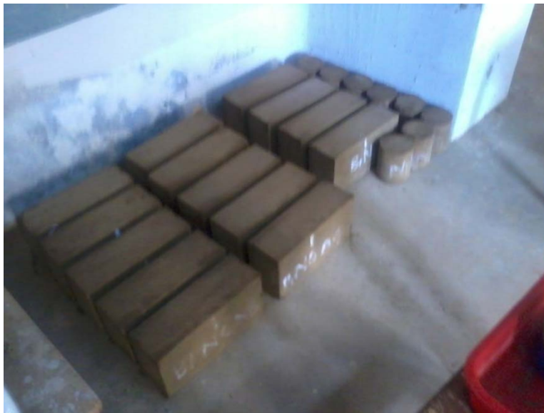
Fig 3.6 (e) Masonry blocks ready for Curing
