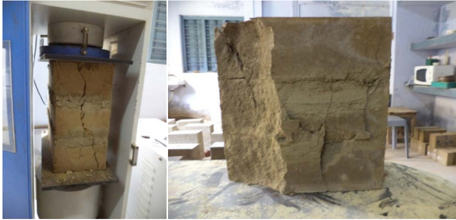
Fig 4.32 Failure of masonry prism (blocks without Kit fibre)
