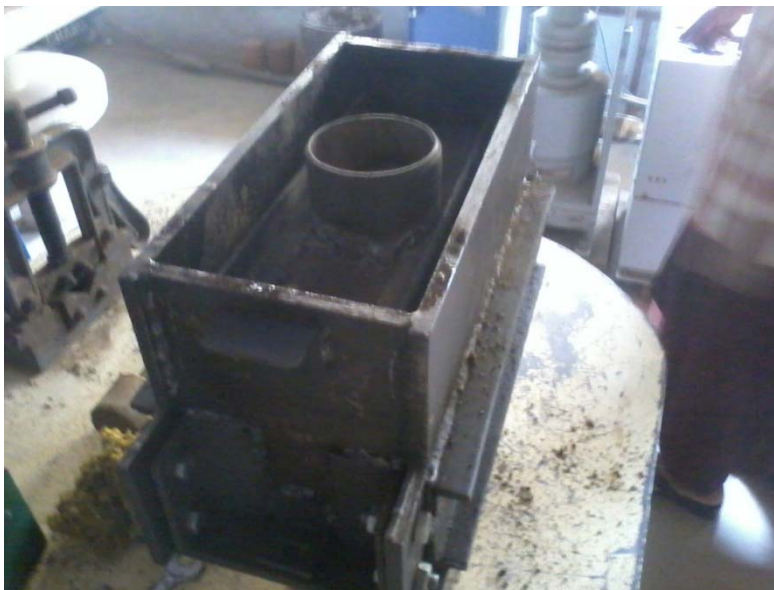
Fig 3.6(c) Filled mould with collar ready for compression
