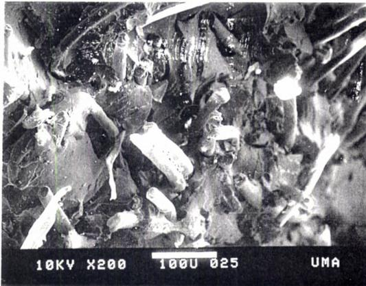
5.11.a. SEM photomicrographs of tensile fracture surface of mix C4 (Fibers in the longitudinal direction)
