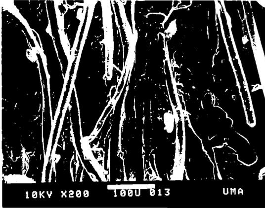
5.12.b. SEM photomicrographs of tensile fracture surface of mix C1 (Fibers in the transverse direction)
