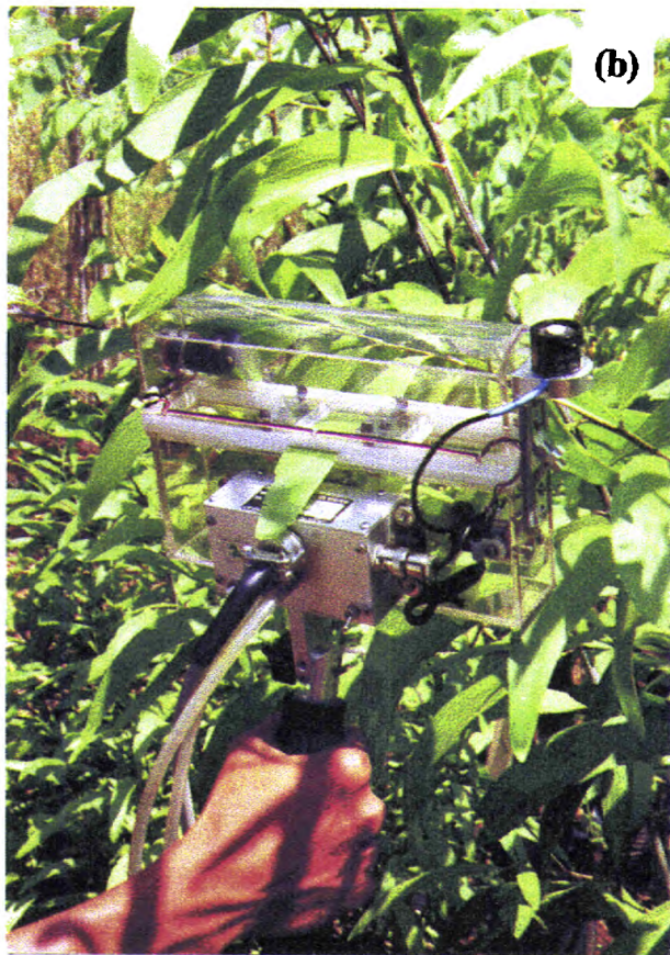
Plate.2. (a) Measurement of water potential using pressure chamber (b) a phyllode of A.auriculiformis in the leaf chamber of the photosynthesis system. (c) a phyllode of A.holocericea in the leaf chamber of steady state porometer
