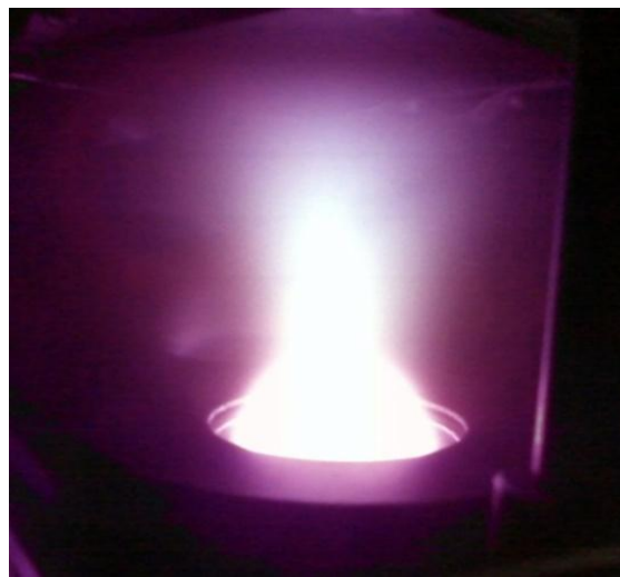
Fig. 3.7: Photograph of the high frequency (27.12MHz) sputtering plasma of \text{LiMn}_2\text{O}_4 target.
