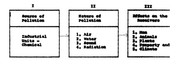
dispersion of pollutants from the source through air, water and land. The third component in the system is the effect of pollution on the receivers namely man, emissis, plants property and climate.
