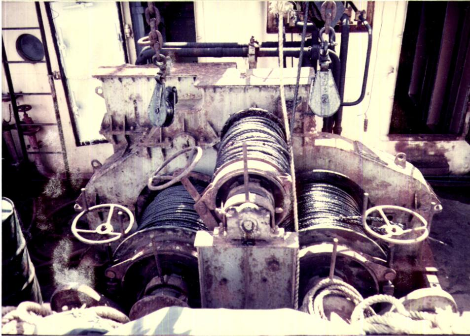
Fig 22. Three drum winch Vessels A, B & C
