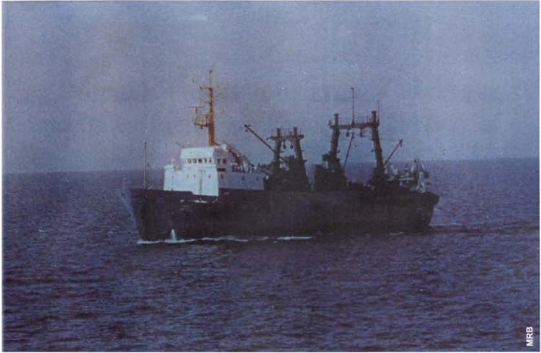
Fig 6.7 62.2 m L_{OA} , 1898 GRT, 2400 hp Intermediate Range Freezer Trawler
