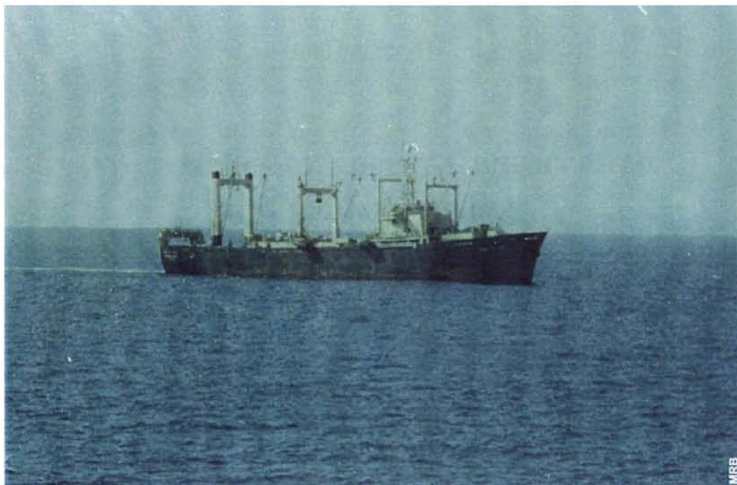
Fig 7.7 110 m L OA , 5460 GRT, 5700 hp Japanese factory trawler
