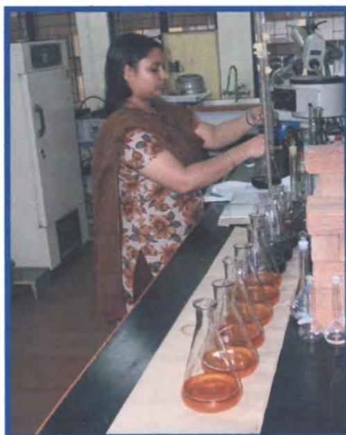
**Fig. 4.2.** Wet oxidation method (Walkley and Black, 1934)
