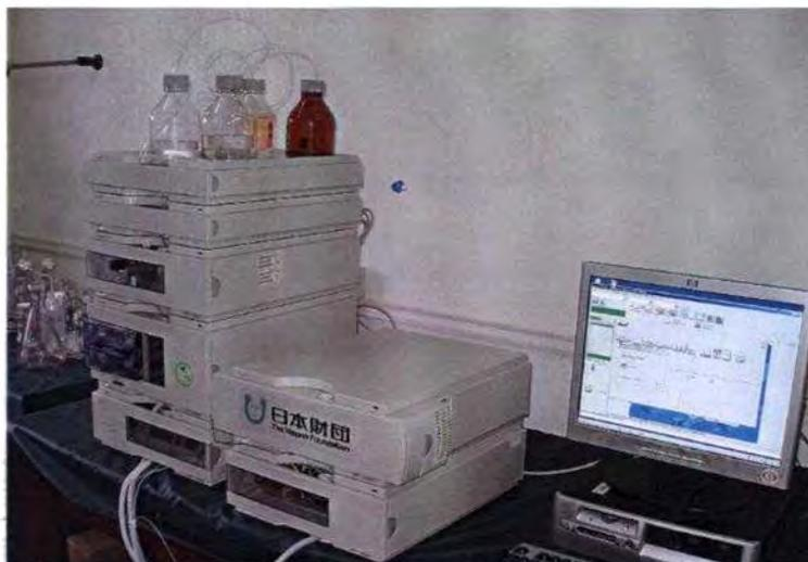
Plate 2.8. High Performance Liquid Chromatography (HPLC)
