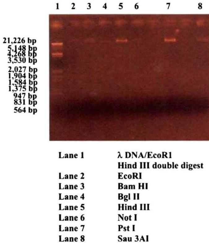
**Fig. 4.25 Restriction pattern of  $\Phi$ MV- 5 phage DNA**
