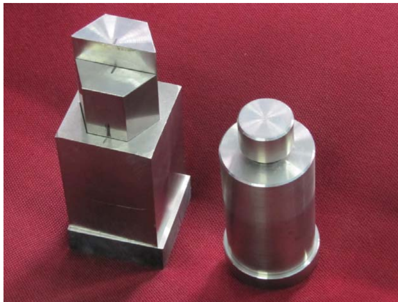
Figure 3.7.3.1: Photograph of Dies used for ITDR and Cylindrical DR
