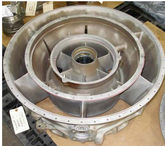
Figure 2.2: ZE41 Mg fan housing in aerospace application [65]
