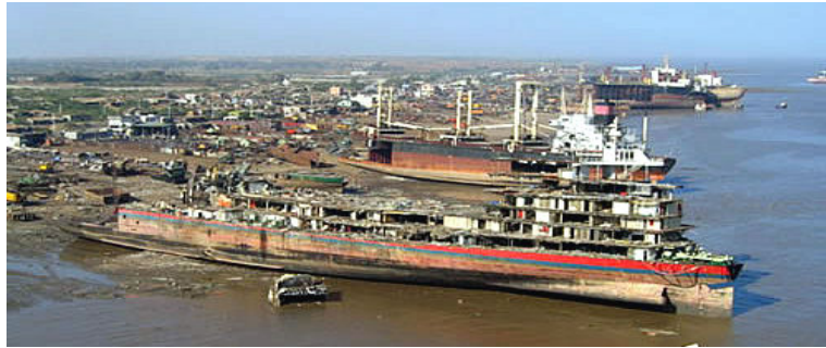
Fig. 2.2 Obsolete Ships Beached for Dismantling ( Sibal 2001)
