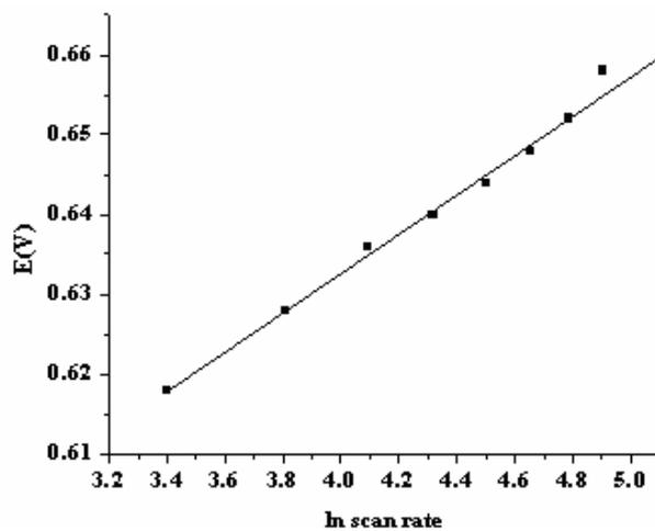
**Figure 7.18** Plot of peak potential against ln (scan rate) at poly (p-ABSA)/GCE
