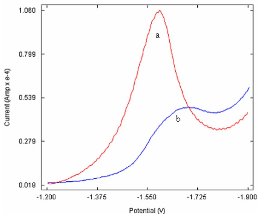
**Figure 6.6** Overlay of Square Wave Voltammogram of LAM at (a) poly (L-Cys) modified GCE and (b) bare GCE at a scan rate of  $0.06\text{Vs}^{-1}$  from  $-1.2 - -1.8\text{ V}$
