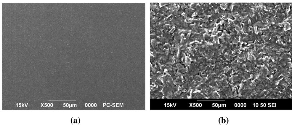
**Figure 7.4** SEM images of (a) bare GCE and (b) poly (p-ABSA)/GCE
