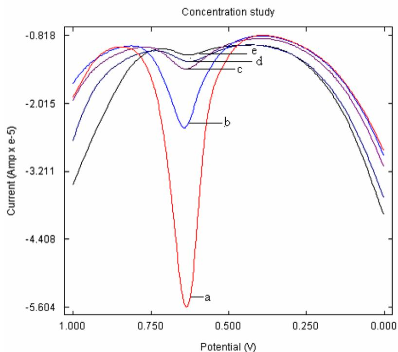
Figure 5.13 Square Wave Voltammogram of PAM Chloride of different concentrations a)  $1 \times 10^{-3} \text{M}$  b)  $1 \times 10^{-4} \text{M}$  c)  $1 \times 10^{-5} \text{M}$  d)  $1 \times 10^{-6} \text{M}$  e)  $1 \times 10^{-7} \text{M}$  at poly (p-TSA) modified GCE at  $25^\circ \text{C}$
