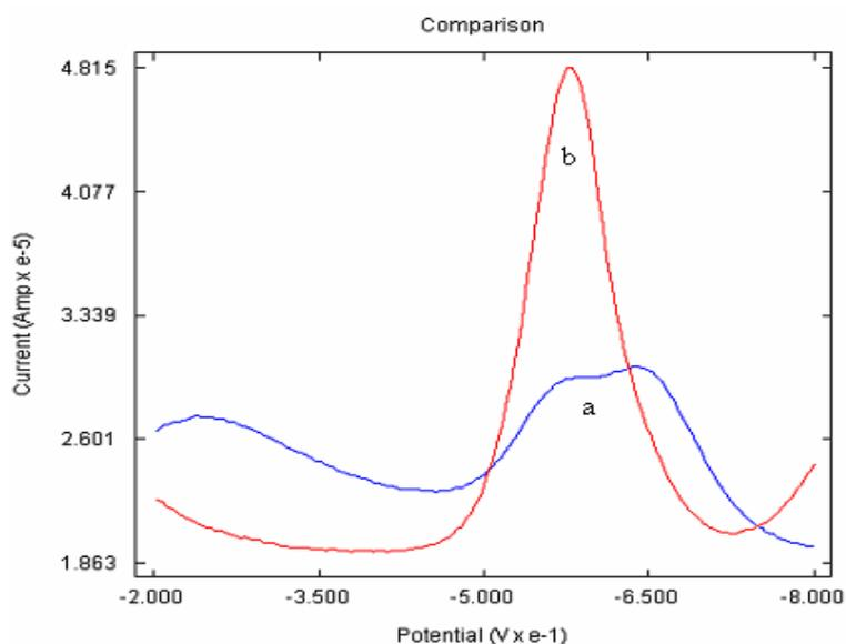
**Figure 8.9** Overlay of Square Wave Voltammogram of NIM at (a) bare GCE (b) AuNP/poly-CA/GCE at a scan rate of  $0.06\text{Vs}^{-1}$  from  $-0.2\text{V}$  to  $-0.8\text{V}$
