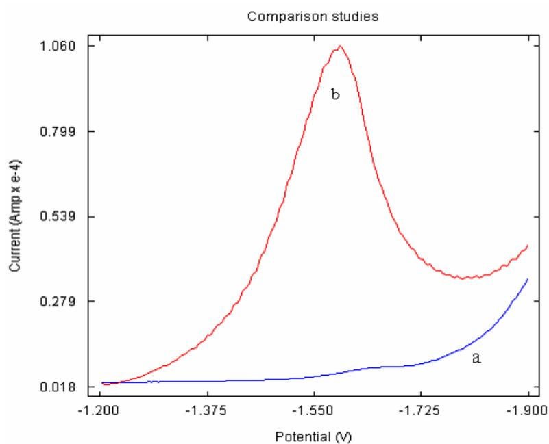
**Figure 6.5** Square Wave Voltammogram showing the voltammetric behaviour of poly (L-Cys) /GCE in PBS pH 7 and without (a) LAM with (b) LAM at a scan rate of  $0.06\text{Vs}^{-1}$  from  $-1.2\text{ V} - -1.8\text{ V}$ .
