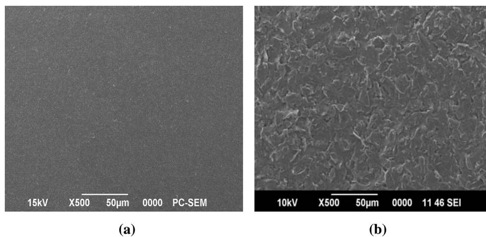
**Figure 6.4** SEM images of (a) bare GCE and (b) poly (L-Cys) modified GCE
