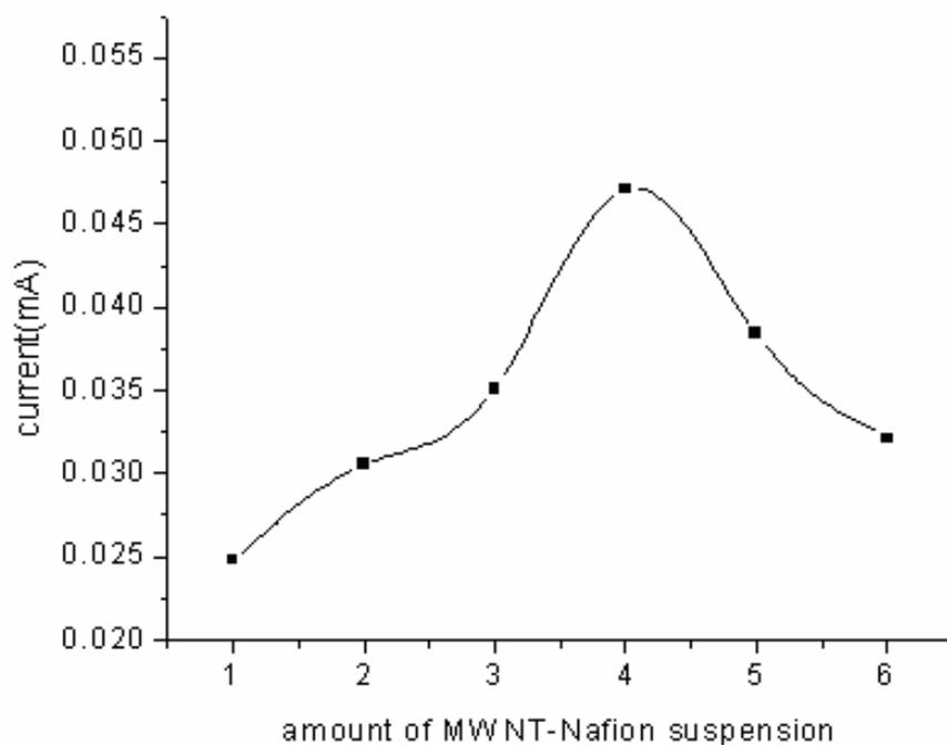
Figure 4.4 Effect of the amount of MWCNT-Nafion suspension.
