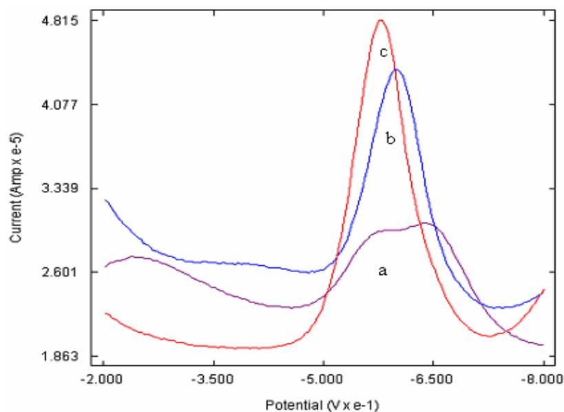
**Figure 8.11** Overlay of Square Wave Voltammograms of NIM at (a) bare GCE (b) poly -CA/GCE and (c) AuNP/ poly-CA/GCE at a scan rate of  $0.06\text{Vs}^{-1}$  from -0.2V to -0.8 V
