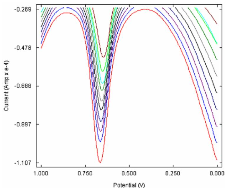
**Figure 5.10** Overlay of SWVs of PAM Chloride at poly (p-TSA)/GCE in 0.1M phosphate buffer (pH 7) containing  $1 \times 10^{-3}$ M PAM Chloride at different scan rates a) 40 b) 60 c) 80 d) 100 e) 120 f) 140 g) 160 h) 180 i) 200  $\text{mVs}^{-1}$ .
