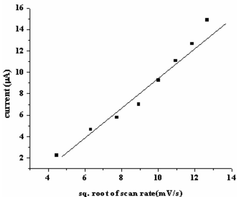
**Figure 8.16** Effect of scan rate at poly-CA/GCE
