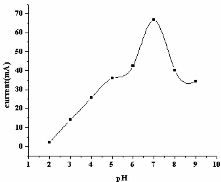
**Figure 5.9** Effect of pH on the anodic peak current of  $1 \times 10^{-3}$ M PAM Chloride
