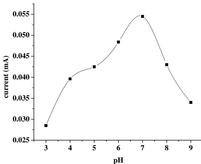
**Figure 7.12** Effect of pH on the cathodic peak current of  $1 \times 10^{-3}$  M MBZ at poly (p-ABSA)/GCE
