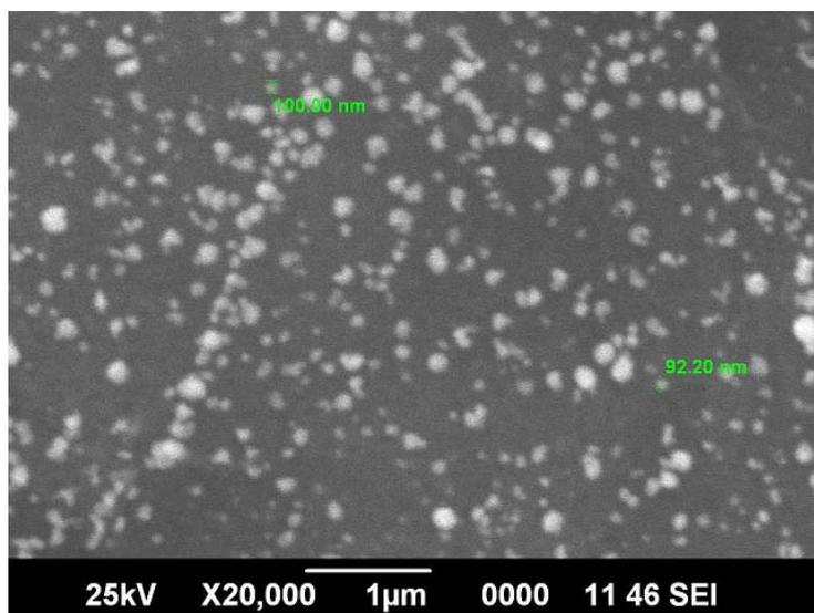
**Figure 8.7 (b)** SEM image of AuNP/poly-CA/GCE showing the size of AuNPs
