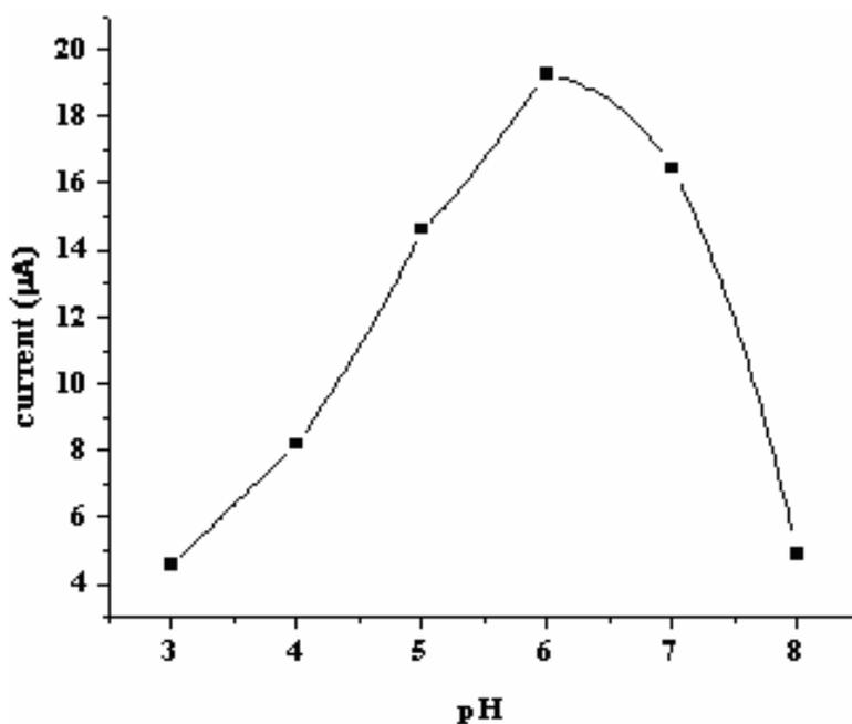
**Figure 8.12** Effect of pH on the cathodic peak current of  $1 \times 10^{-4}\text{M}$  NIM at poly- CA/GCE
