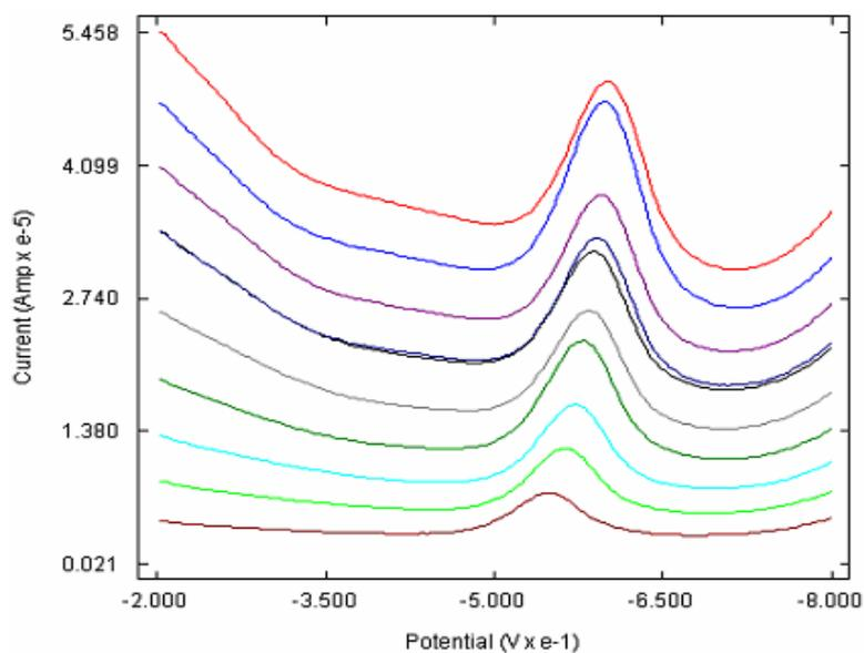
**Figure 8.15** Overlay of SWVs of NIM at AuNP/poly -CA/GCE in 0.1M phosphate buffer (pH 6) containing  $1 \times 10^{-4}$  M NIM at different scan rates a) 20 b) 40 c) 60 d) 80 e) 100 f) 120 g) 140 h) 160 i) 180 j)  $200 \text{ mVs}^{-1}$ .
