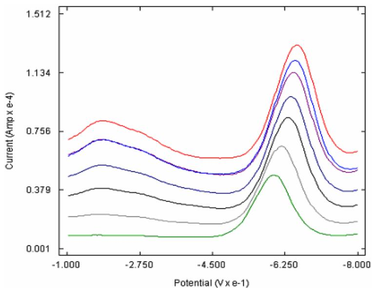
**Figure 7.14** Overlay of SWVs of MBZ at poly (p-ABSA)/GCE in 0.1M phosphate buffer (pH 7) containing  $1 \times 10^{-3}$ M MBZ at different scan rates a) 30 b) 45 c) 60 d) 75 e) 90 f) 105 g) 120 h) 135  $\text{mVs}^{-1}$ .
