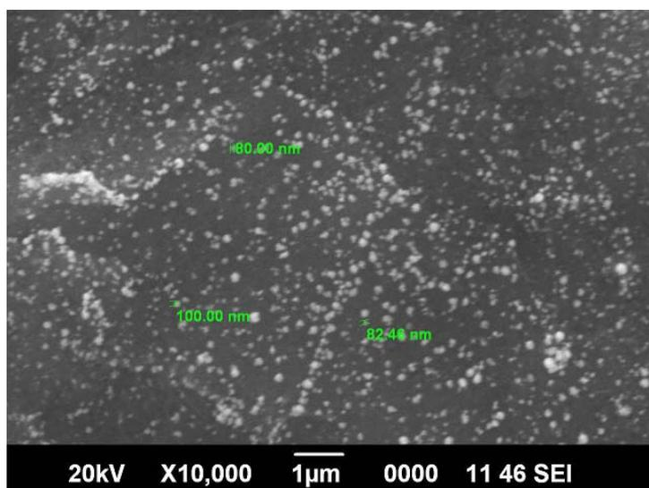
**Figure 7.7(b)** SEM image of AuNP/poly (p-ABSA)/GCE showing the size of AuNPs
