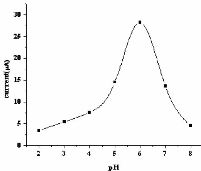
**Figure 8.13** Effect of pH on the cathodic peak current of  $1 \times 10^{-4}$  M NIM at AuNP/ poly- CA/GCE
