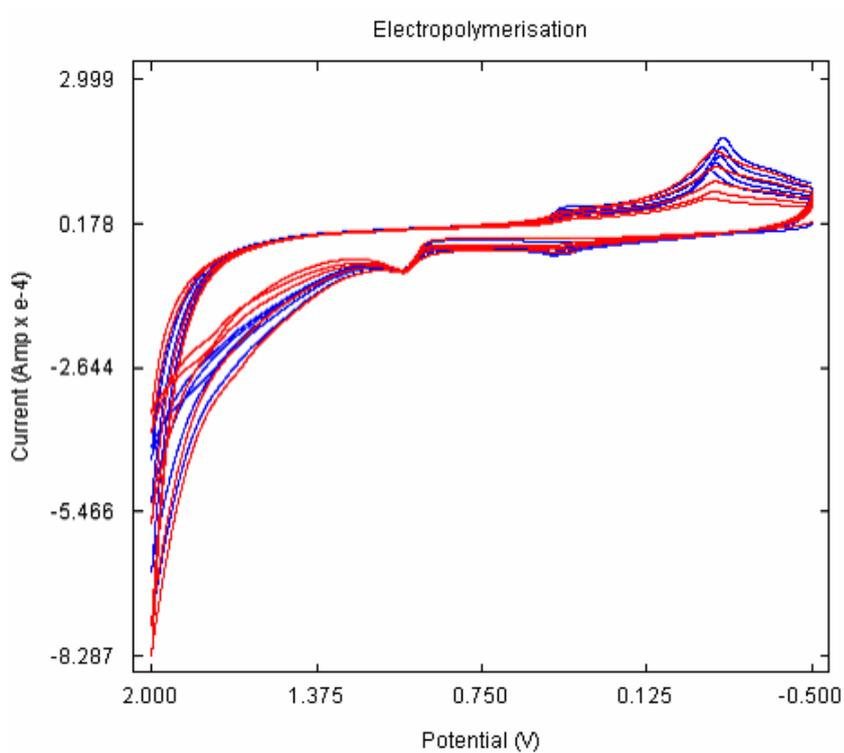
**Figure 7.2** Electropolymerization of p-ABSA at GCE
