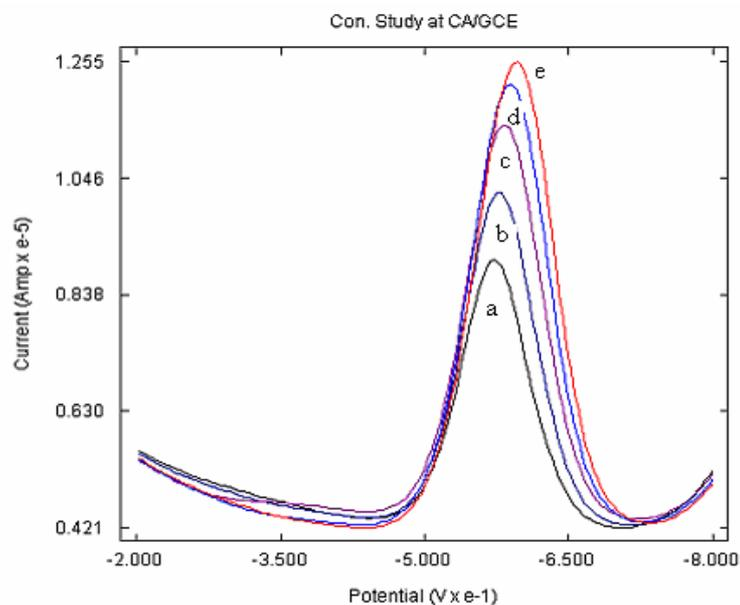
**Figure 8.21** Differential Pulse Voltammogram of NIM of different concentrations a)  $1 \times 10^{-5}$  M b)  $3 \times 10^{-5}$  M c)  $5 \times 10^{-5}$  M d)  $7 \times 10^{-5}$  M e)  $1 \times 10^{-4}$  M at poly-CA/GCE at  $25^{\circ}\text{C}$
