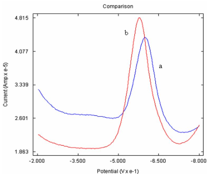
**Figure 8.10** Overlay of Square Wave Voltammogram of NIM at (a) poly-CA/GCE (b) AuNP/poly-CA/GCE at a scan rate of  $0.06\text{Vs}^{-1}$  from  $-0.2\text{V}$  to  $-0.8\text{V}$
