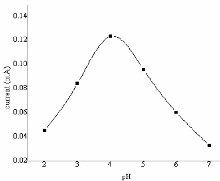
**Figure 3.5** Effect of pH on the oxidation peak current of AMB
