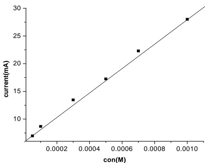
**Figure 6.13** Calibration curve for LAM at poly (L-Cys) modified GCE at  $25^{\circ}\text{C}$
