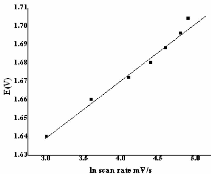
Figure 6.11 Plot of peak potential against ln (scan rate)
