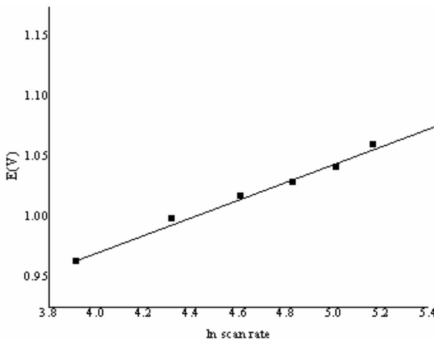
Figure 3.9 Plot of peak potential against ln (scan rate)
