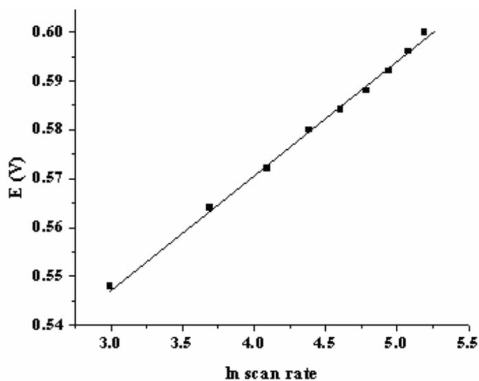
Figure 8.19 Plot of peak potential against ln (scan rate) at AuNP /poly-CA/GCE
