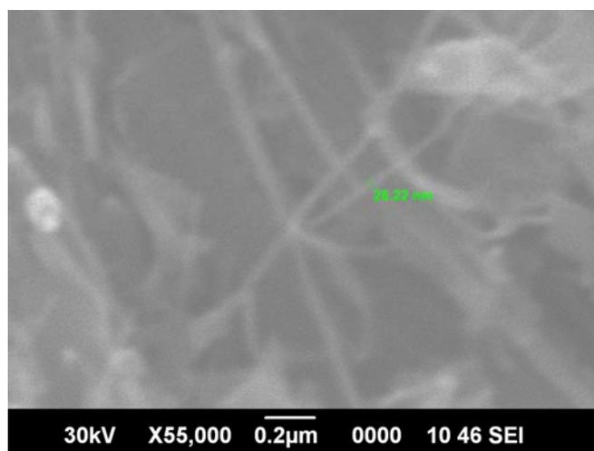
**Figure 3.2** SEM image of MWCNT after acid treatment.
