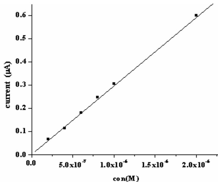
**Figure 5.14.** Calibration curve for PAM Chloride at poly (p-TSA) modified GCE at 25<sup>0</sup>C
