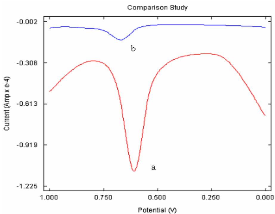
**Figure 5.5** Overlay of Square Wave Voltammogram of PAM Chloride at (a) poly (p-TSA) modified GCE and (b) bare GCE at a scan rate of  $0.06\text{Vs}^{-1}$  from 0 – 1.0 V
