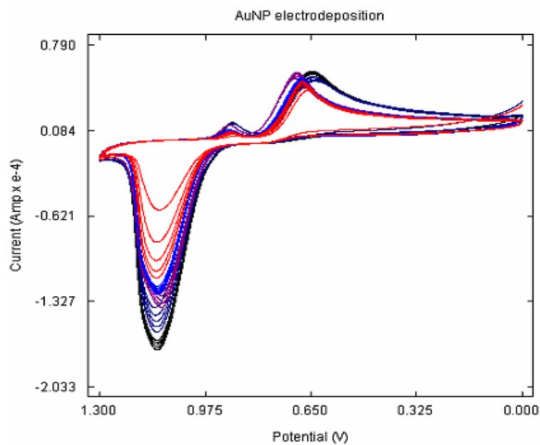
**Figure 7.5** Electrodeposition of AuNP at poly(p-ABSA)/GCE
