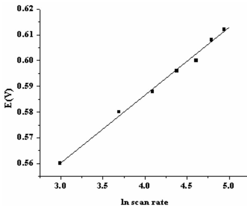
Figure 8.18 Plot of peak potential against ln (scan rate) at poly-CA/GCE
