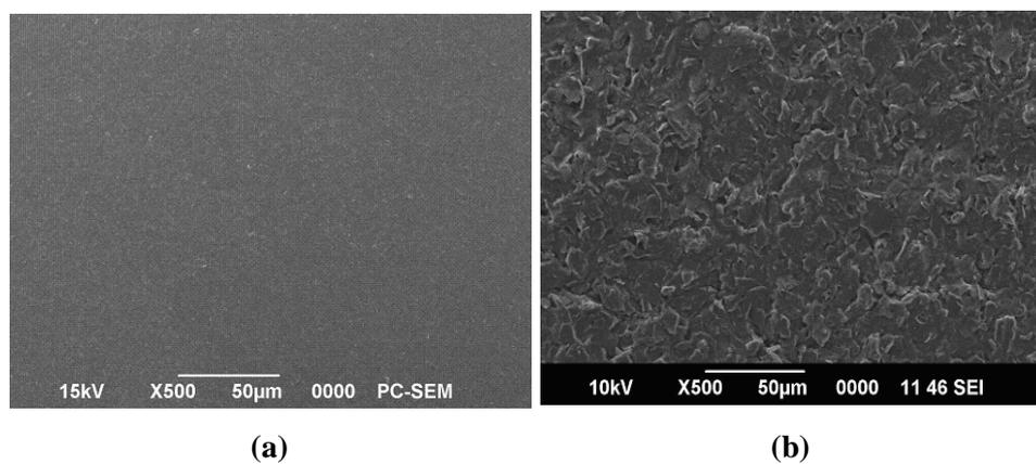
**Figure 8.4** SEM images of (a) bare GCE and (b) poly -CA/GCE
