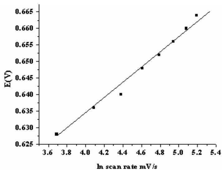
Figure 5.12 Plot of peak potential against ln (scan rate)
