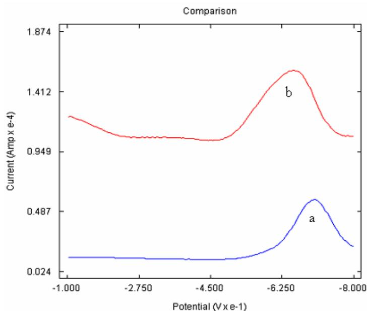
**Figure 7.8** Overlay of Square Wave Voltammogram of MBZ at (a) bare GCE (b) poly (p-ABSA)/GCE at a scan rate of  $0.06\text{Vs}^{-1}$  from  $-0.1\text{V}$  to  $-0.8\text{V}$
