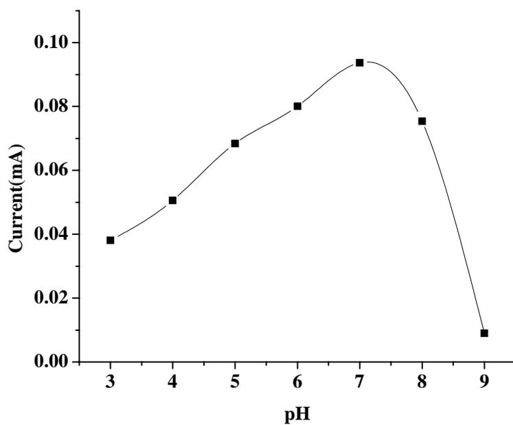
**Figure 7.11** Effect of pH on the cathodic peak current of  $1 \times 10^{-3}$  M MBZ at AuNP/ poly (p-ABSA)/GCE
