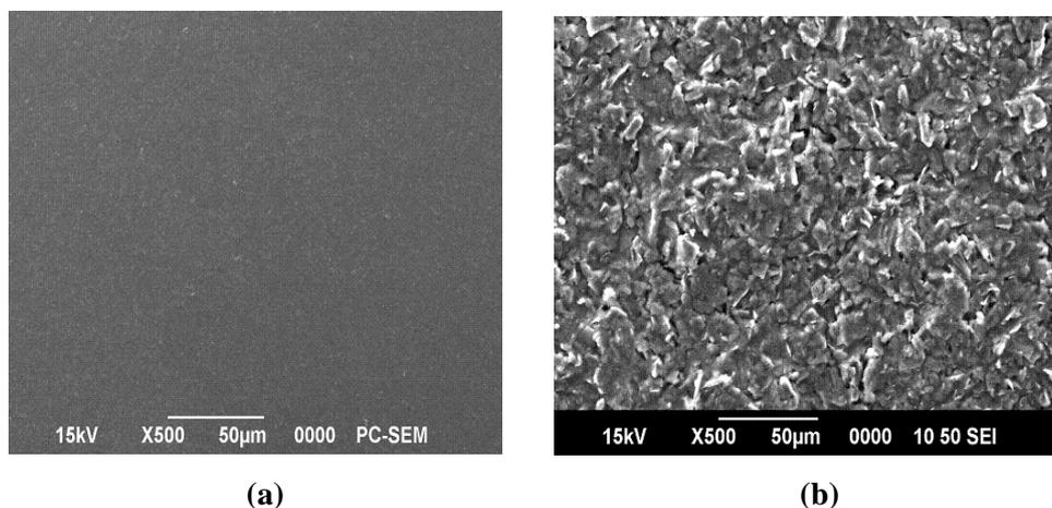
**Figure 5.3** SEM images of (a) bare GCE and (b) poly (p-TSA) modified GCE
