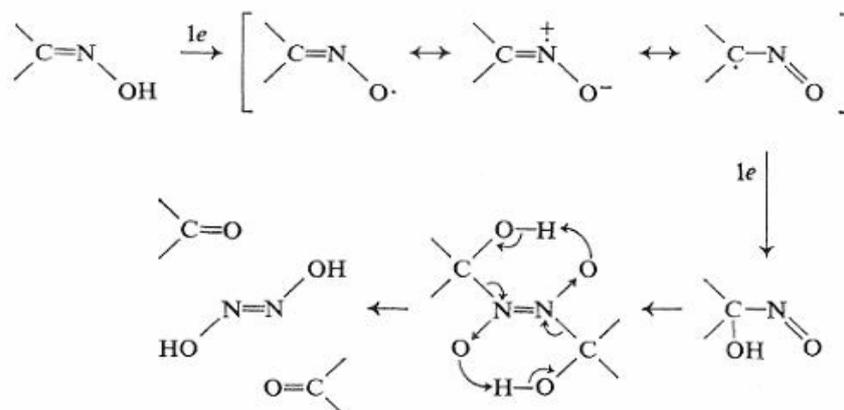
**Figure 5.7** Mechanism of oxidation of oxime group in PAM Chloride to carbonyl group
