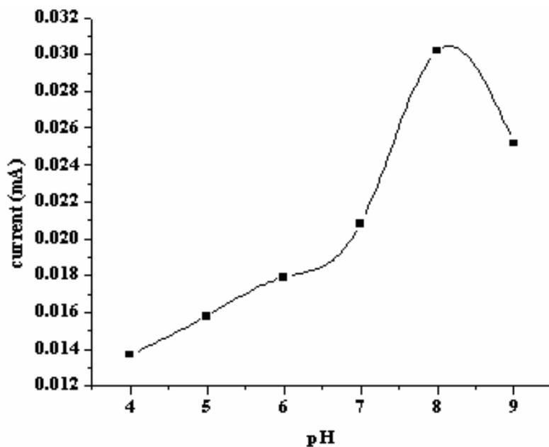
Figure 4.3 Effect of pH on the anodic current of  $1 \times 10^{-3}$  M SMX.
