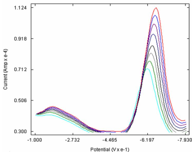
**Figure 7.13** Overlay of SWVs of MBZ at AuNP/poly (p-ABSA)/GCE in 0.1M phosphate buffer (pH 7) containing  $1 \times 10^{-3}$ M MBZ at different scan rates a) 30 b) 45 c) 60 d) 75 e) 90 f) 105 g) 120 h) 135  $\text{mVs}^{-1}$ .
