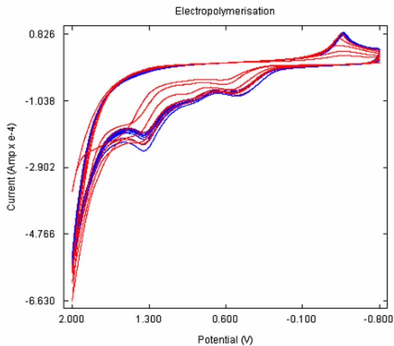
**Figure 6.2** Electropolymerization of L-Cys at GCE
