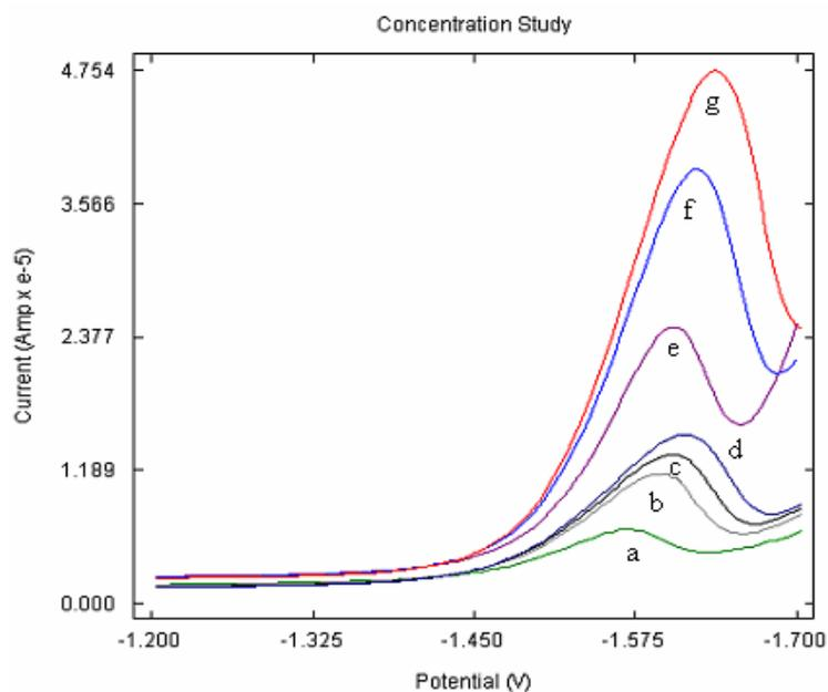
**Figure 6.12** Differential Pulse Voltammogram of LAM of different concentrations a)  $1 \times 10^{-5}$  M b)  $3 \times 10^{-5}$  M c)  $5 \times 10^{-5}$  M d)  $7 \times 10^{-5}$  M e)  $1 \times 10^{-4}$  M f)  $3 \times 10^{-4}$  M g)  $5 \times 10^{-4}$  M at poly (L-Cys) modified GCE at  $25^{\circ}\text{C}$
