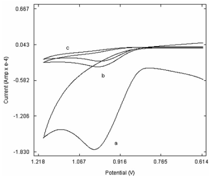
**Figure 3.4** Cyclic Voltammogram of AMB at (a) MWCNT/ Nafion / GCE (b) Nafion/GCE and (c) bare GCE
