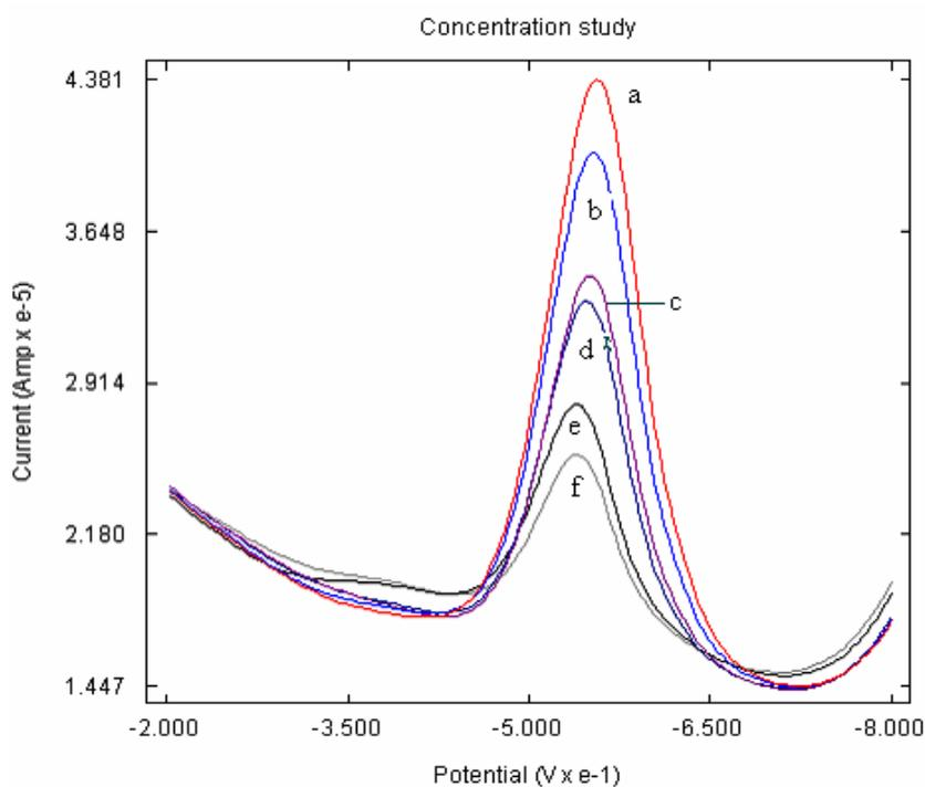
**Figure 7.20** Differential Pulse Voltammogram of MBZ of different concentrations a)  $1 \times 10^{-5}$ M b)  $8 \times 10^{-6}$ M c)  $5 \times 10^{-6}$ M d)  $2 \times 10^{-6}$ M e)  $8 \times 10^{-7}$ M f)  $4 \times 10^{-7}$ M at AuNP/poly (p-ABSA) modified GCE at  $25^{\circ}\text{C}$
