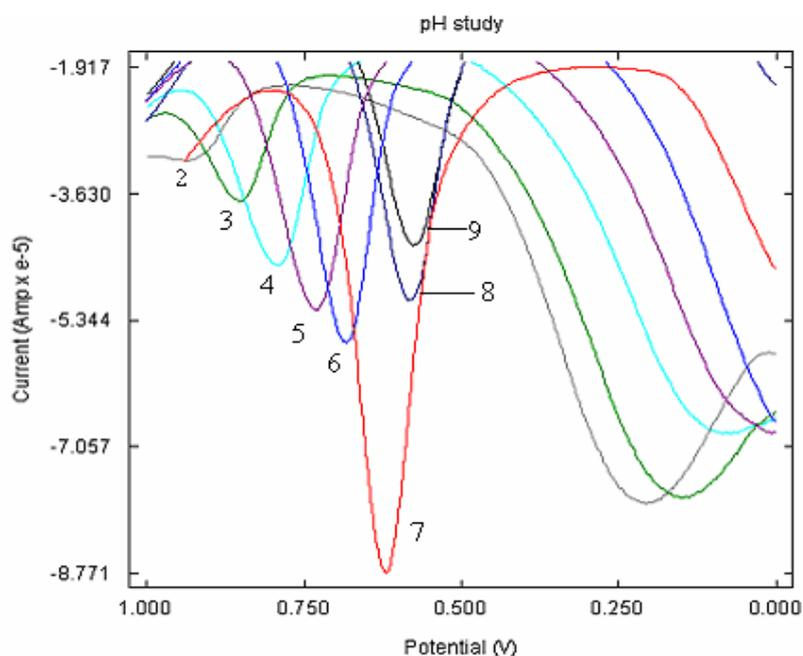
**Figure 5.8** Overlay of SWVs of PAM Chloride at poly (p-TSA)/GCE in 0.1M phosphate buffer containing  $1 \times 10^{-3}$ M PAM Chloride at different pH 2, 3, 4, 5, 6, 7, 8 and 9.
