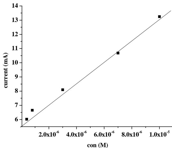
**Figure 7.21** Calibration curve for MBZ at AuNP/poly (p-ABSA)/GCE at 25<sup>0</sup>C
