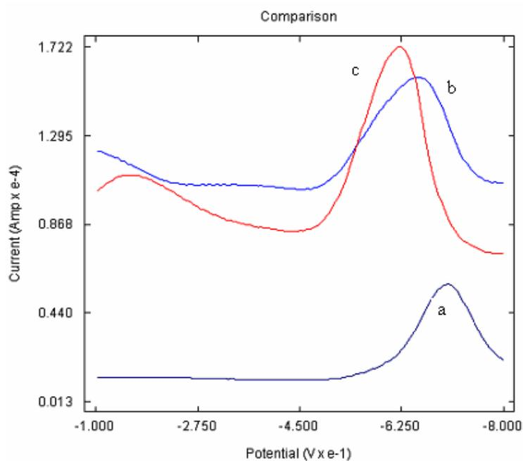
**Figure 7.10** Overlay of Square Wave Voltammograms of MBZ at (a) bare GCE (b) poly (p-ABSA)/GCE and (c) AuNP/poly (p-ABSA)/GCE at a scan rate of  $0.06\text{Vs}^{-1}$  from -0.1V to -0.8 V
