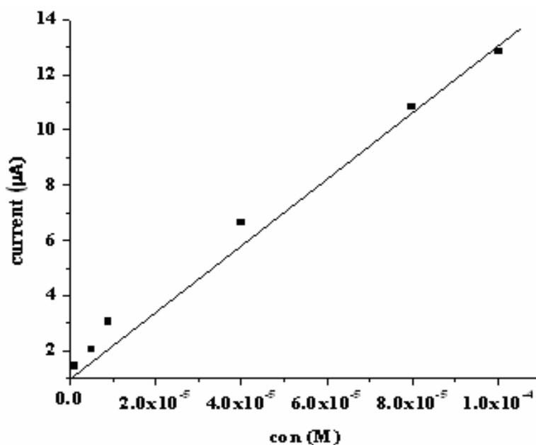
**Figure 8.24** Calibration curve for NIM at AuNP/poly-CA/GCE at  $25^{\circ}\text{C}$
