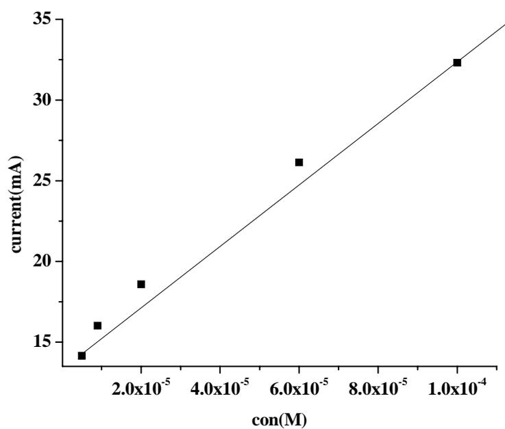
**Figure 7.23** Calibration curve for MBZ at poly (p-ABSA)/GCE at 25<sup>0</sup>C
