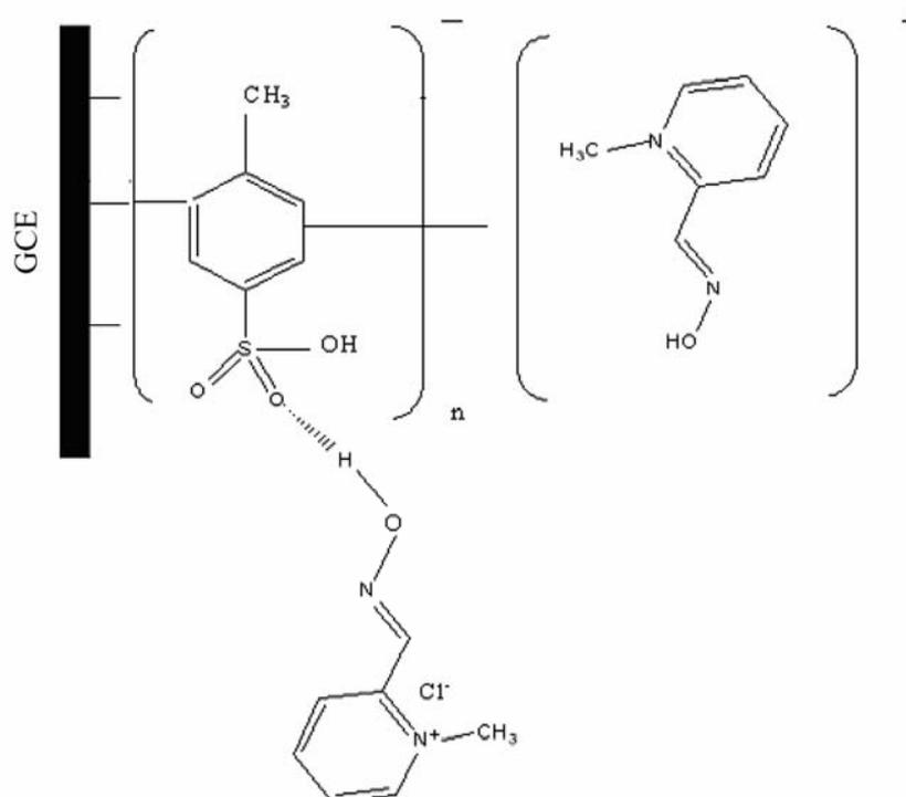
**Figure 5.6** Electropolymerization of p-TSA at GCE and the attachment of PAM Chloride at this modified surface
