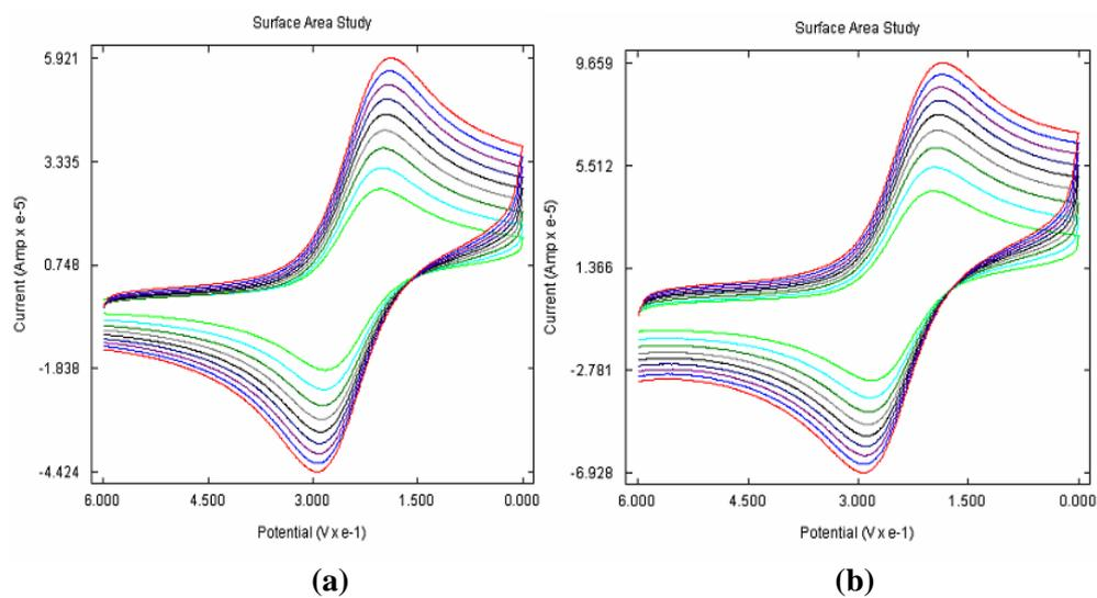
**figure 6.3** Surface area study at a) bare GCE and b) poly (L-Cys)/GCE
