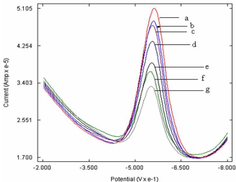
**Figure 7.22** Differential Pulse Voltammogram of MBZ of different concentrations a) 1x10<sup>-4</sup>M b) 6x10<sup>-5</sup>M c) 2x10<sup>-5</sup>M d) 9x10<sup>-6</sup>M e) 7x10<sup>-6</sup>M f) 5x10<sup>-6</sup>M at poly (p-ABSA) modified GCE at 25<sup>0</sup>C
