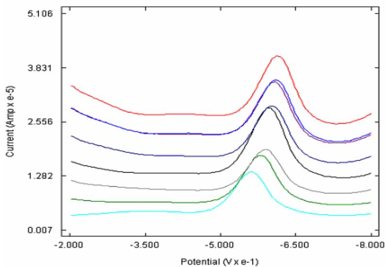
**Figure 8.14** Overlay of SWVs of NIM at poly -CA/GCE in 0.1M phosphate buffer (pH 6) containing  $1 \times 10^{-4}$  M NIM at different scan rates a) 20 b) 40 c) 60 d) 80 e) 100 f) 120 g) 140 h) 160  $\text{mVs}^{-1}$ .
