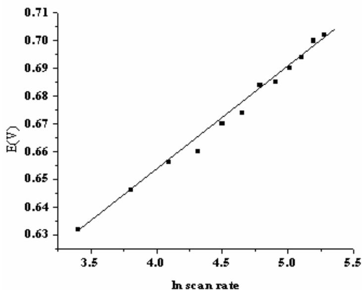
**Figure 7.17** Plot of peak potential against ln (scan rate) at AuNP / poly(p-ABSA)/GCE
