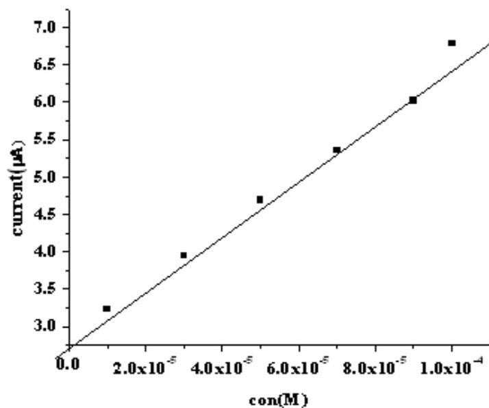
**Figure 8.22** Calibration curve for NIM at poly-CA/GCE at  $25^{\circ}\text{C}$
