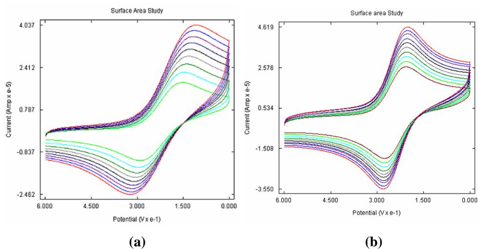
**Figure 8.3** Surface area study at a) bare GCE and b) poly- CA/GCE
