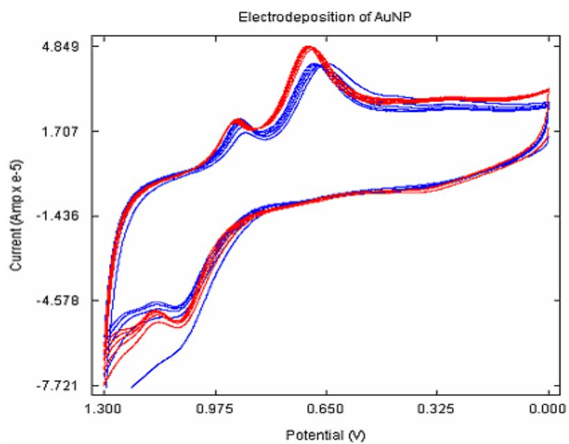
**Figure 8.5** Electrodeposition of AuNP at poly-CA/GCE
