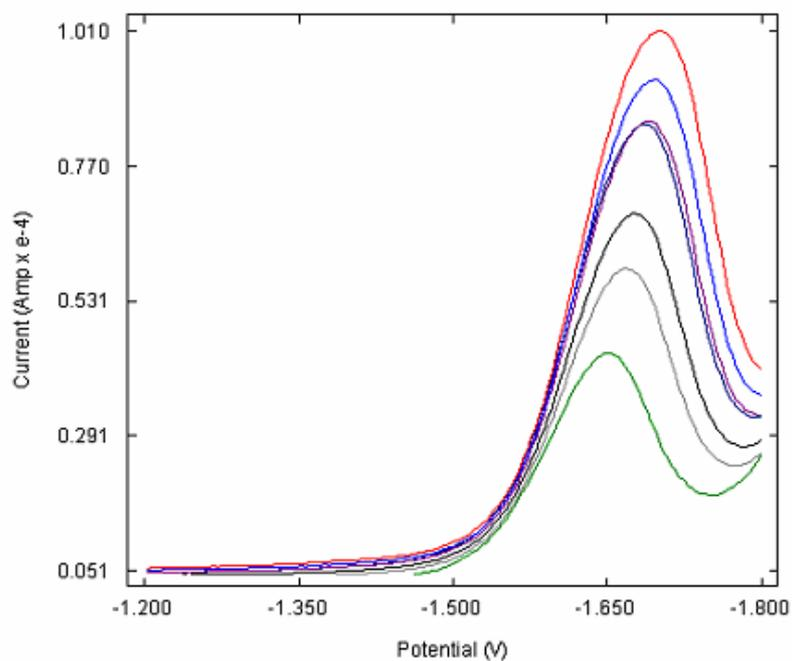
**Figure 6.9** Overlay of SWVs of LAM at poly (L-Cys)/GCE in 0.1M phosphate buffer (pH 7) containing  $5 \times 10^{-3}$  M LAM at different scan rates a) 40 b) 60 c) 80 d) 100 e) 120 f) 140 g) 160  $\text{mVs}^{-1}$ .
