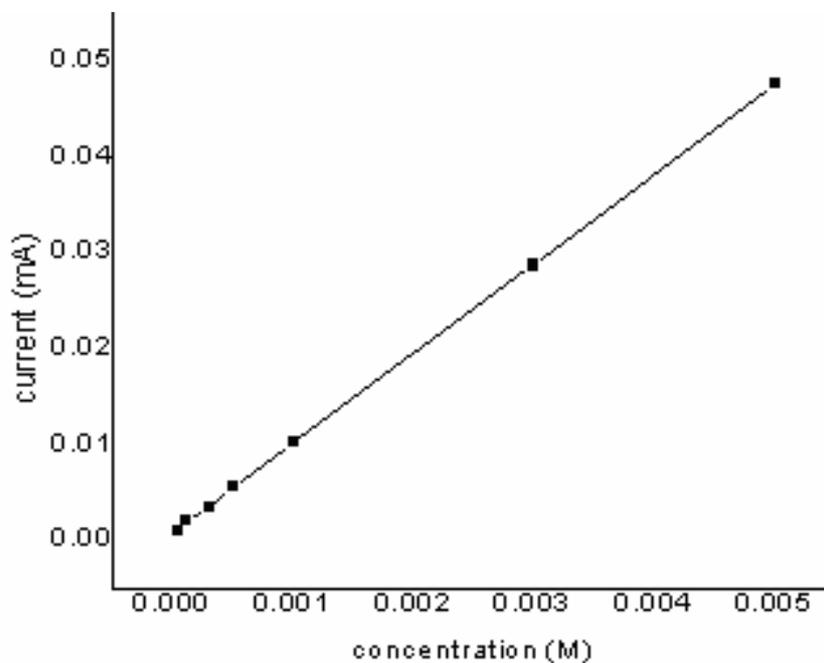
**Figure 4.6** Calibration graph for SMX at MWCNT modified GCE at 25<sup>0</sup>C
