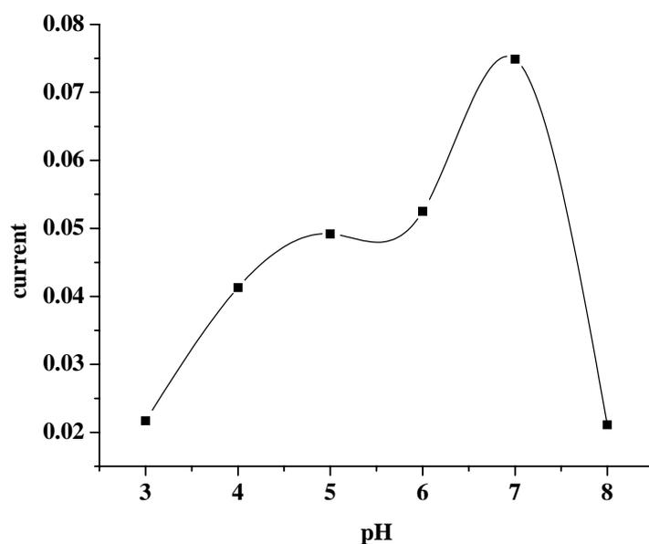
**Figure 6.8** Effect of pH on the cathodic peak current of  $5 \times 10^{-3}$  M LAM
