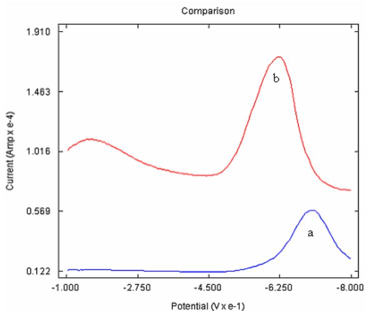
**Figure 7.9** Overlay of Square Wave Voltammogram of MBZ at (a) bare GCE (b) AuNP/poly (p-ABSA)/GCE at a scan rate of  $0.06\text{Vs}^{-1}$  from  $-0.1\text{V}$  to  $-0.8\text{V}$
