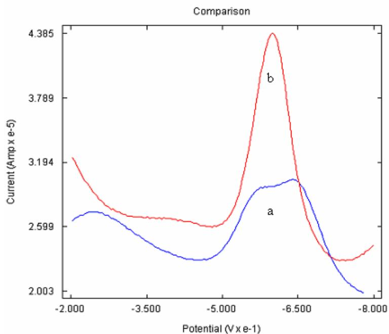
**Figure 8.8** Overlay of Square Wave Voltammogram of NIM at (a) bare GCE (b) poly-CA/GCE at a scan rate of  $0.06\text{Vs}^{-1}$  from  $-0.2\text{V}$  to  $-0.8\text{V}$
