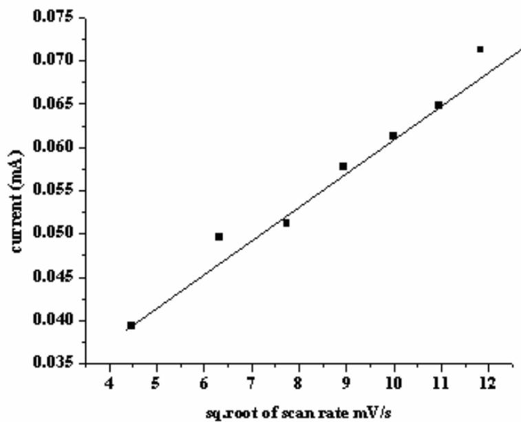
Figure 7.15 Effect of scan rate at AuNP/poly(p-ABSA)/GCE
