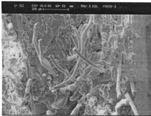
Figure 3.C.2.6e. SEM photomicrograph of tensile fracture surface of mix D with fibers oriented in longitudinal direction (original magnification \times 100 ; marker 200\mu )
