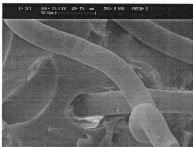
Figure 3.C.2.6d. SEM photomicrograph of tensile fracture surface of mix L with fibers oriented in longitudinal direction (original magnification \times 500 ; marker 50\mu )
