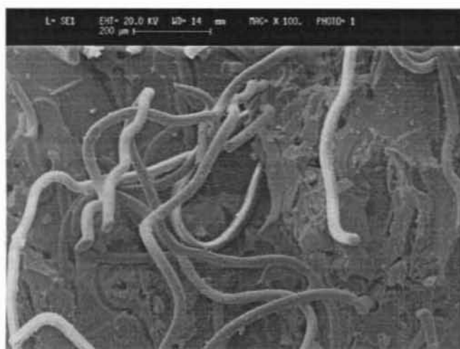
Figure 3.A.2.6f. SEM photomicrograph of tensile fracture surface of mix B with fibers oriented in longitudinal direction (original magnification \times 100 ; marker 200\mu )
