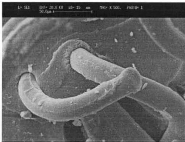
Figure 3.A.2.6e. SEM photomicrograph of tensile fracture surface of mix J with fibers oriented in longitudinal direction (original magnification \times 500 ; marker 50\mu )
