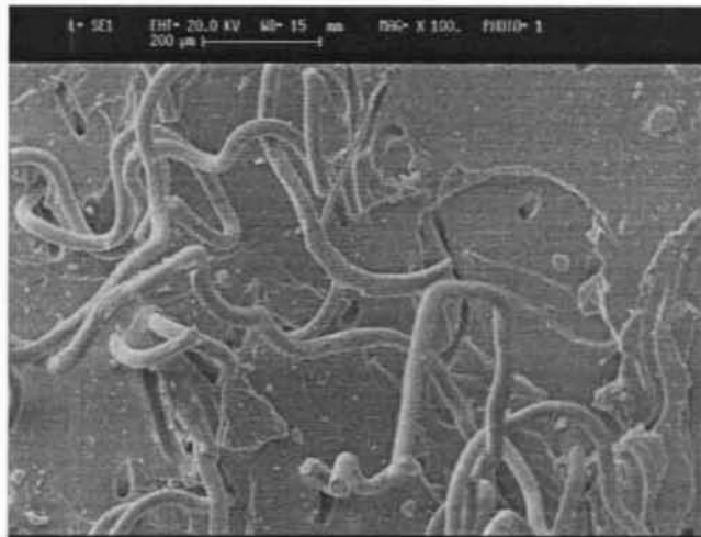
Figure 3.A.2.6d. SEM photomicrograph of tensile fracture surface of mix J with fibers oriented in longitudinal direction (original magnification \times 100 ; marker 200\mu )
