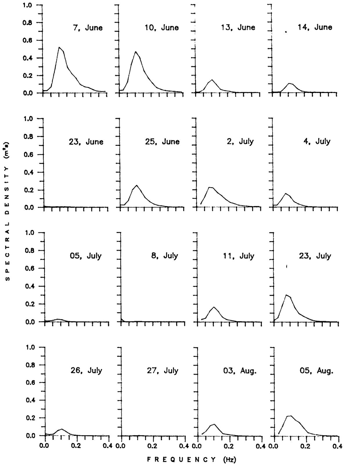
Fig. 4.9 Systematic transformation of nearshore wave spectra during pre-mudbank, mudbank and post-mudbank conditions for 1988.
