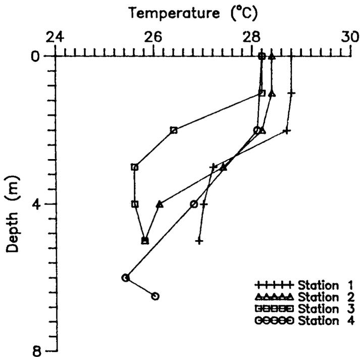
Fig. 5.2 Vertical temperature profiles at different stations during dissipation stages of mudbank
