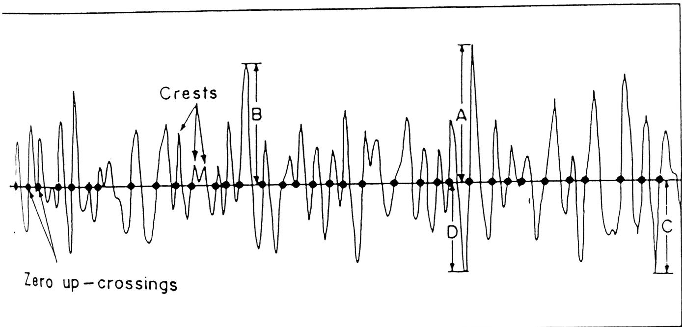
Fig. 3.11 Scheme of Tucker analysis of wave records
