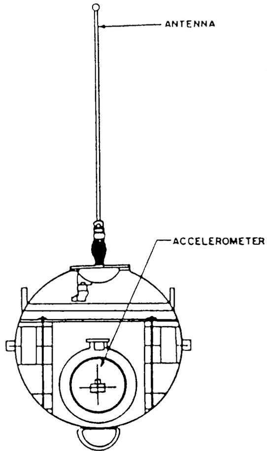
Fig. 3.8 Cross-section of the waverider buoy
