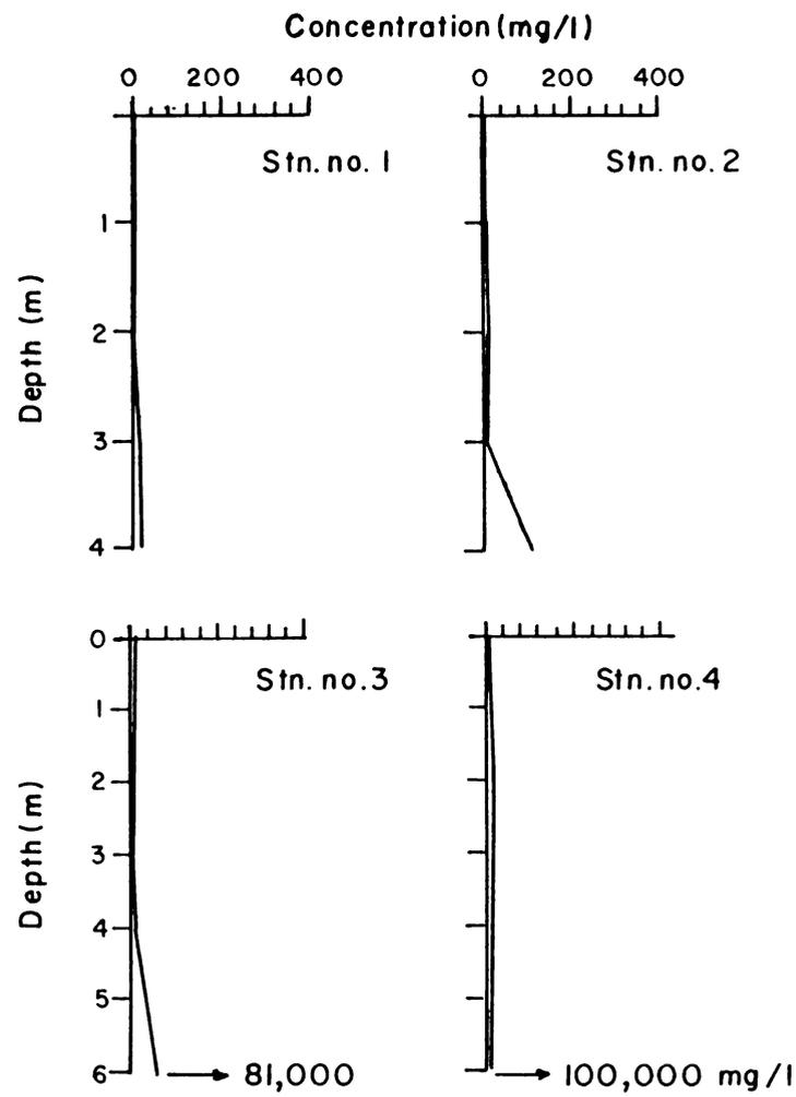
Fig.4.16. Vertical distribution of SSC at different stations in the mudbank (See Fig 3.10 for station locations)
