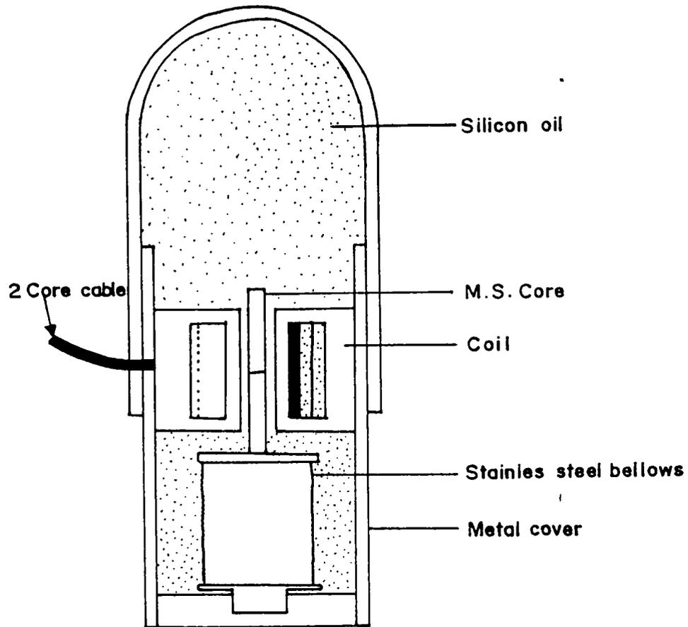
Fig. 3.4 Transducer of wave and tide recorder
