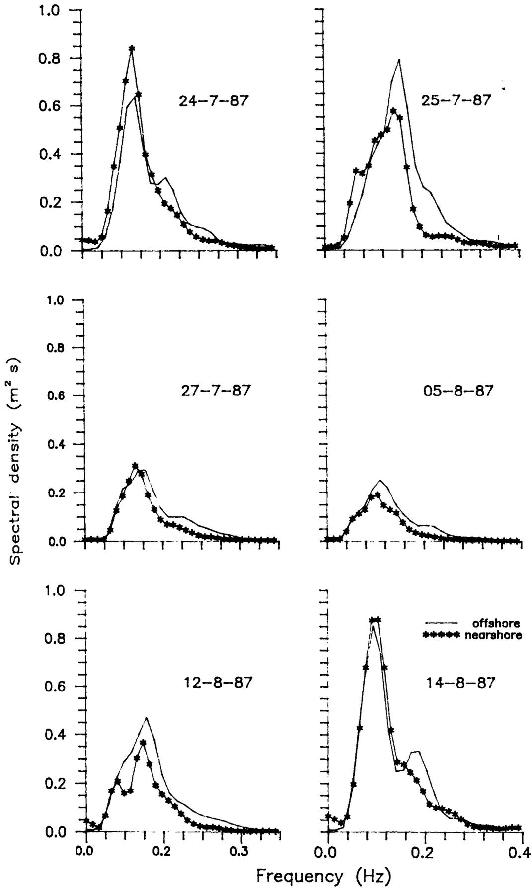
Fig. 4.6 Comparison of synchronous nearshore and offshore wave spectra in the absence of mudbank
