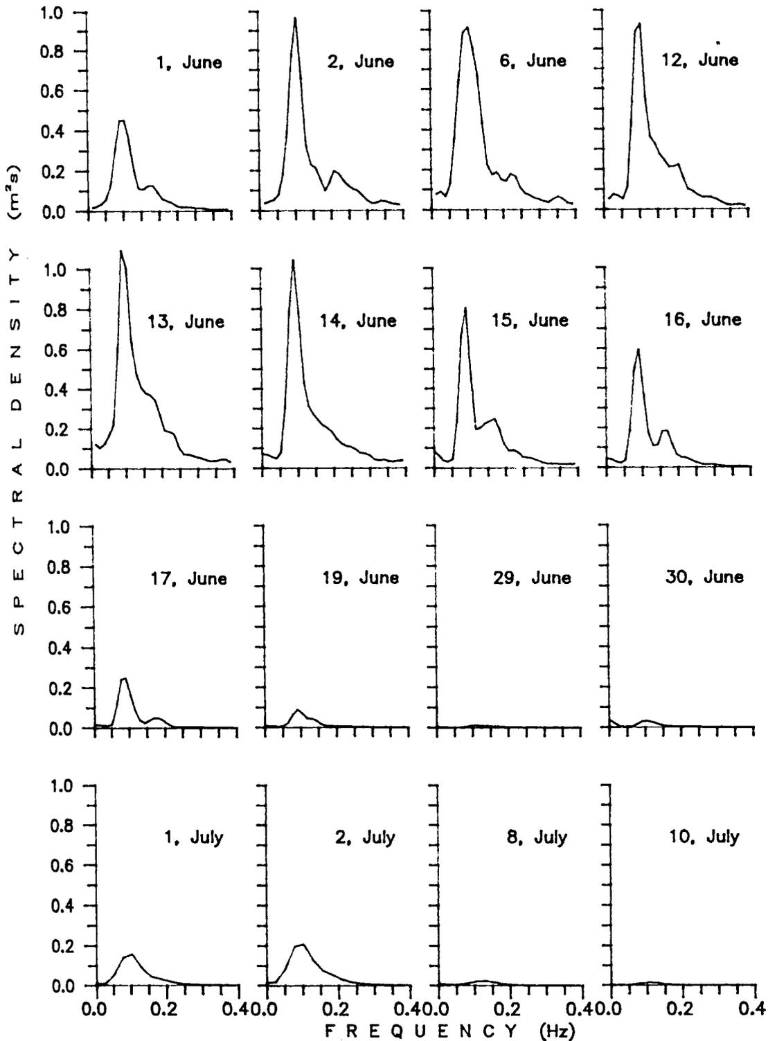
Fig. 4.10 Systematic transformation of nearshore wave spectra during pre-mudbank and mudbank conditions for 1989 (The mudbank dissipated on 20th July due to high wave activity, which damaged even the wave recorder and hence no spectrum could be presented showing the dissipation stage).
