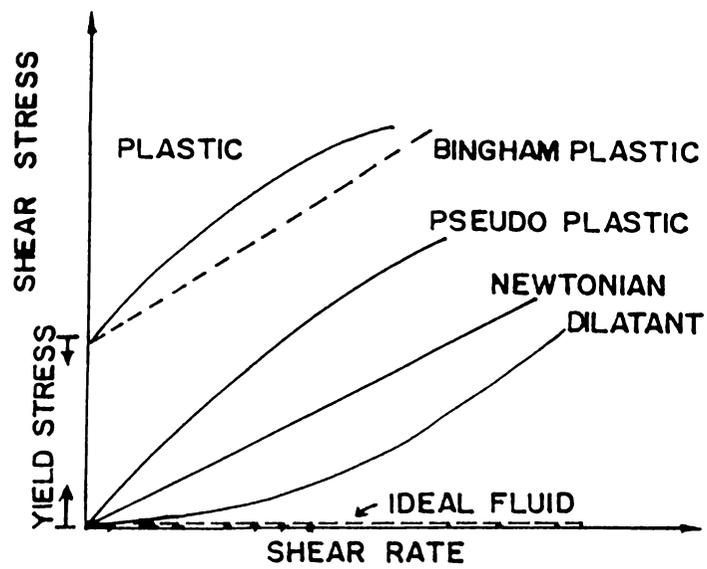
Fig.2.2 . VARIATION OF SHEAR STRESS WITH VELOCITY GRADIENT
