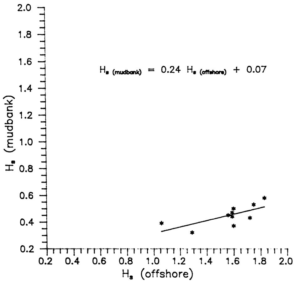
Fig. 4.12 Comparison of synchronous mudbank and offshore (inside & outside the mudbank respectively) significant wave height
