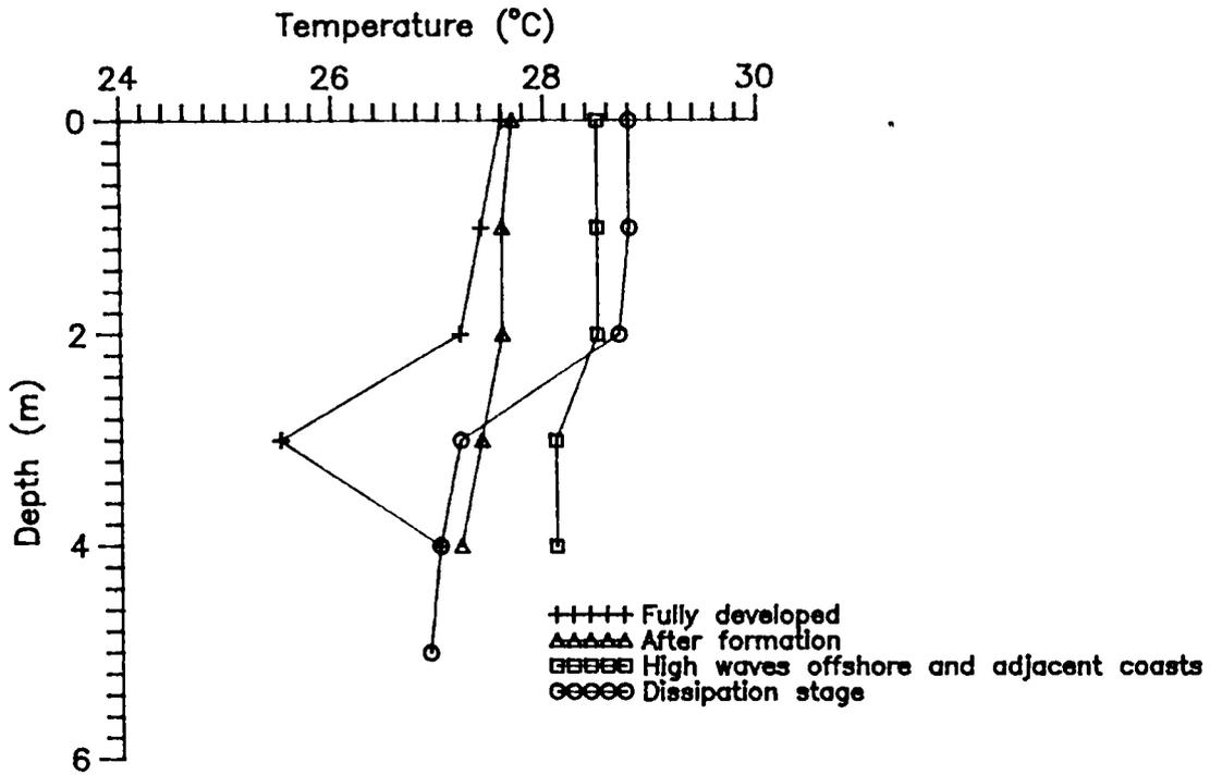
Fig. 5.1 Vertical temperature profiles at different stages of mudbanks
