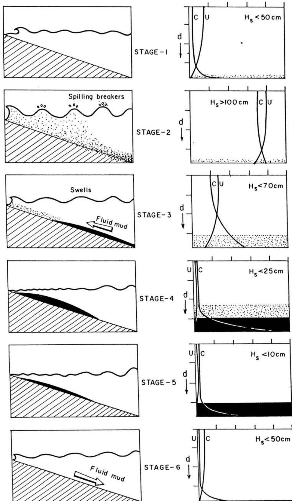
Fig.5.4. Conceptual model of mudbank (C-Concentration, U- Orbital velocity, d - Depth)
