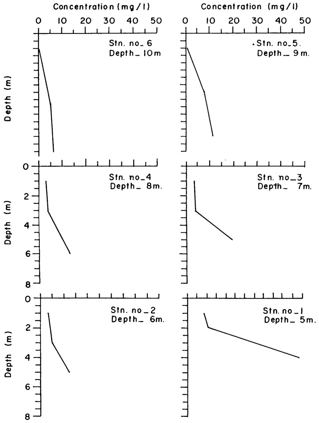
Fig. 4.14. Vertical variation of suspended sediment concentration during non\_mudbank period ( July, 1987). See Fig. 3.10 for station locations.
