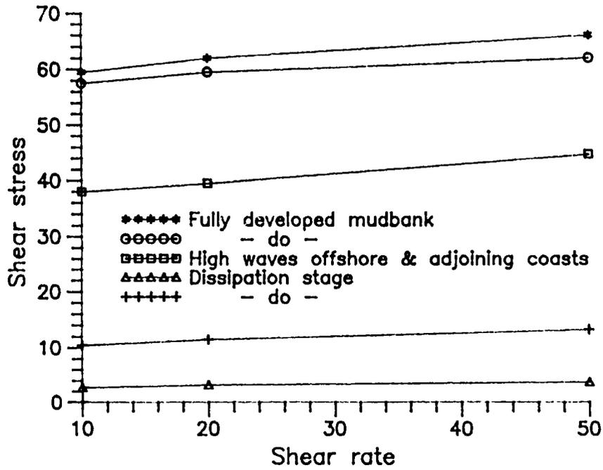
Fig. 4.19 Plot of shear stress vs shear rate during different stages of mudbank
