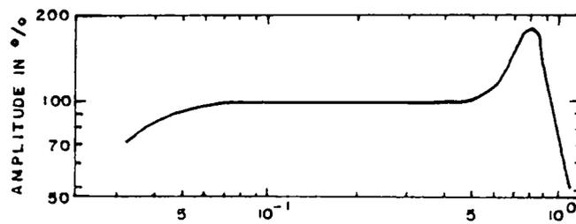
Fig. 3.9 Frequency response of waverider
