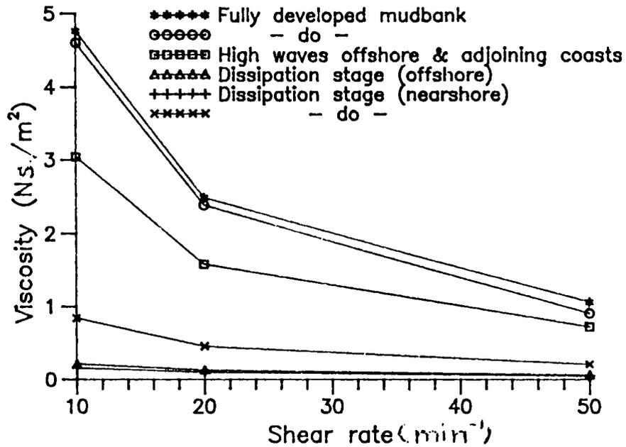
Fig. 4.20 Decrease in viscosity with increase in shear rate
