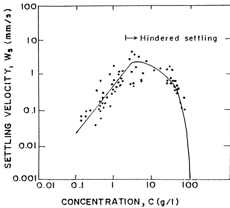
Fig. 2.1 Median settling Velocity Vs. concentration for Severn Estuary Mud ( after Thorn, 1981 ).
