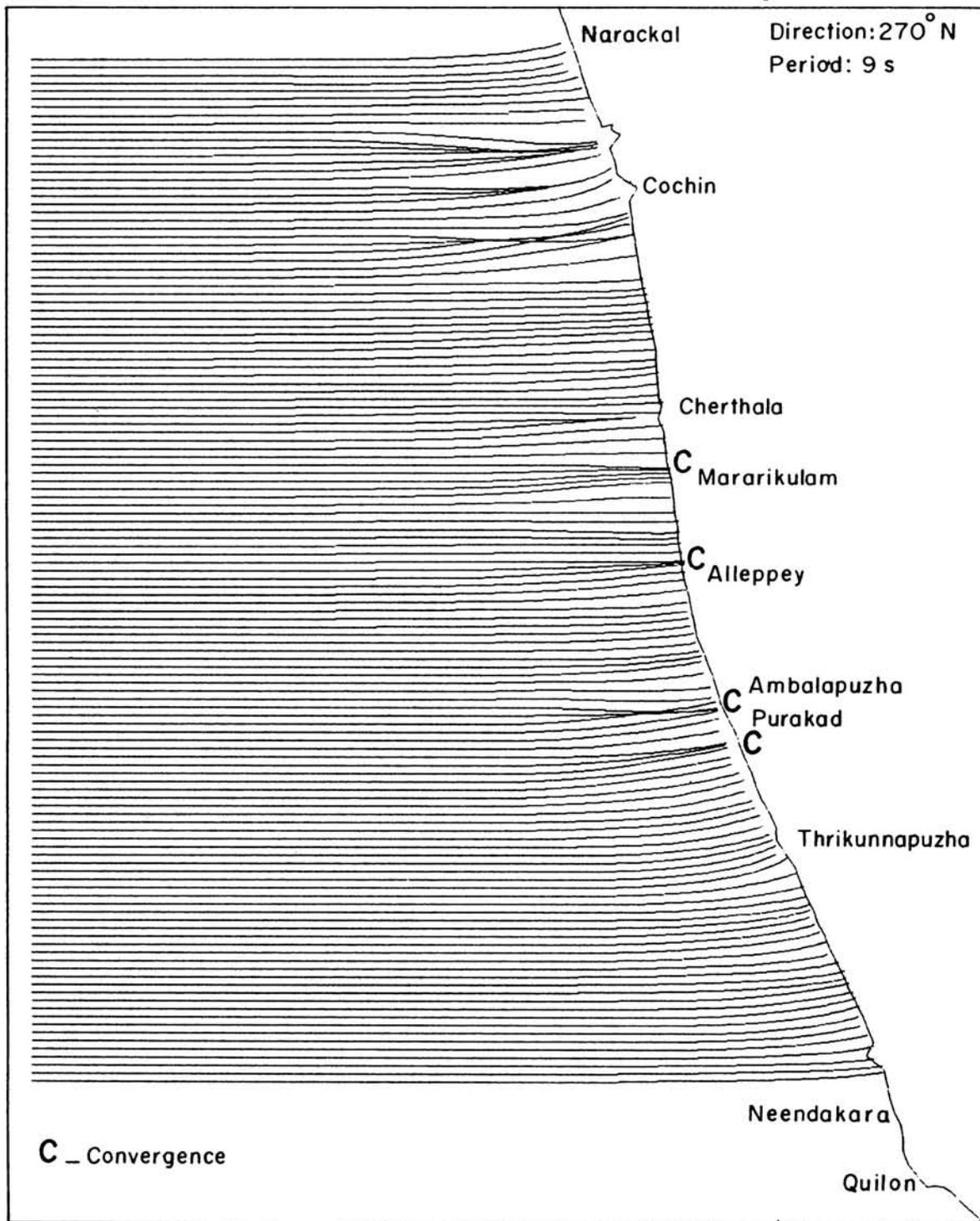
Fig. 5.3 Wave refraction pattern for westerly deep water waves
