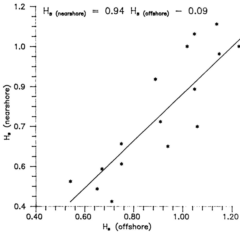
Fig. 4.5 Comparison of synchronous nearshore and offshore significant wave heights in the absence of mudbank
