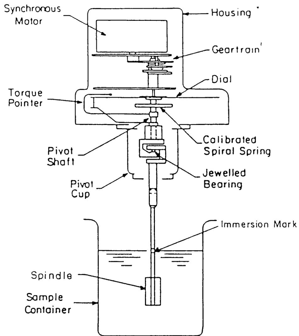
Fig. 3.12 Skeletal structure of Brookfield viscometer
