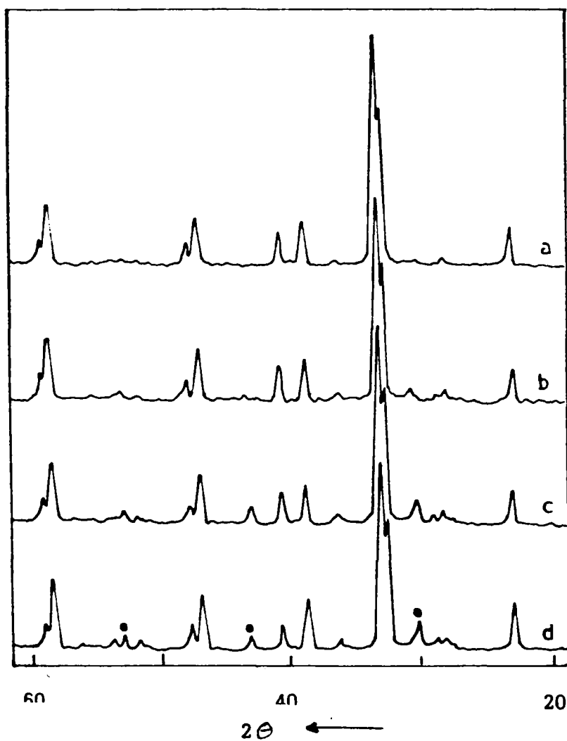
Fig. 3.2: XRD pattern of different wt % of Nb 2 O 5 added YBCO cooled slowly to room temperature in oxygen atmosphere (a) 0 ; (b) 0.5 ; (c) 1.0 ; (d) 2.0 All the samples showed orthorhombic structure with no appreciable variations in lattice parameters.
