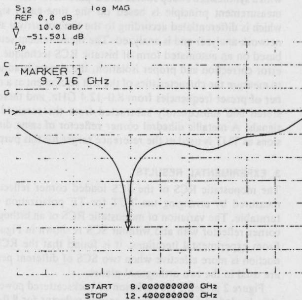
**Figure 2** Variation of backscattered power against the frequency for the corner reflector with and without SCS.  $d_1 = 1.5 + 1.5 \text{ cm.}$   $h = 0.12\lambda$ .  $d_2 = 1.2 + 1.2 \text{ cm.}$   $h = 0.16\lambda$ . Solid line, with SCS; dashed line, without SCS
