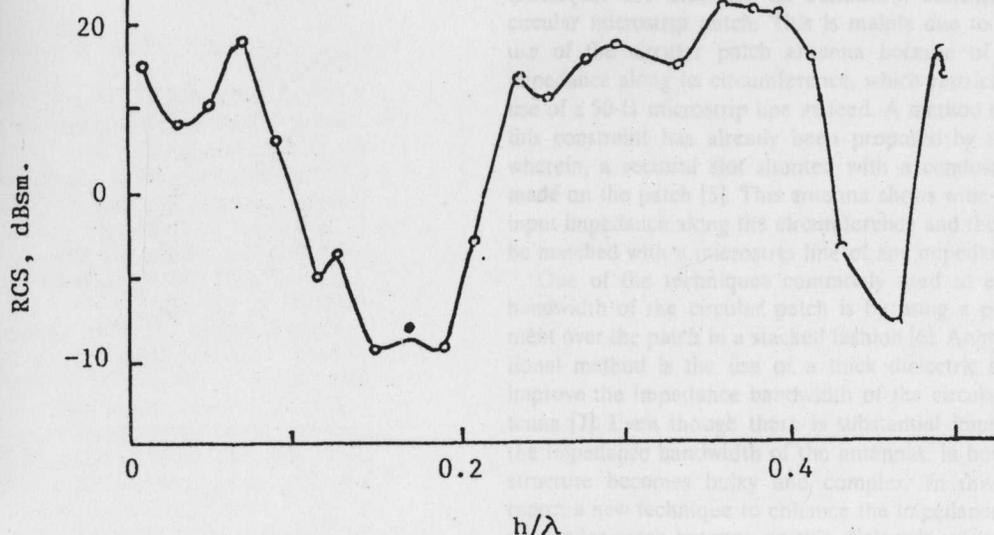
Figure 4 Dependence of the thickness of the dielectric sheet on RCS for corner reflector.  $f = 9.71$  GHz
