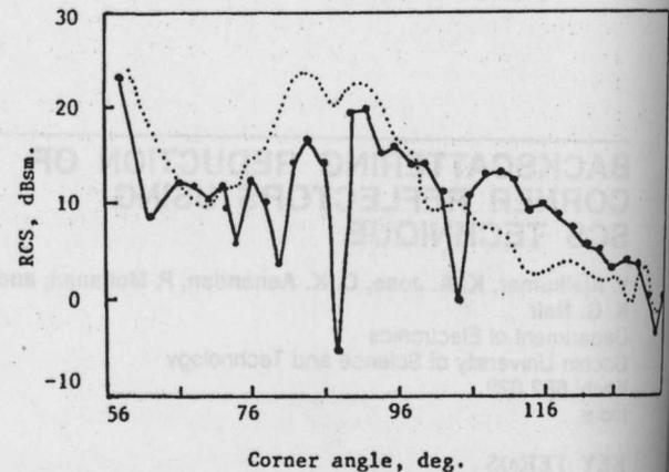
**Figure 3** Variation of RCS against the variation of corner angle  $2\alpha$ .  $f = 9.71 \text{ GHz}$ . Solid line, with SCS; dotted line, without SCS
