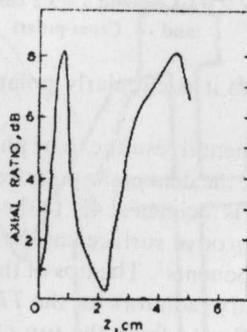
Fig. 2 Variation of axial ratio with the position of the flange from the aperture ( $Z$ ) (Flanges with corrugation parameters  $d = 0.1875\lambda$ ,  $a = 0.156\lambda$ ,  $h = 0.125\lambda$  and flange angle  $2\beta = 45^\circ$ ; horn length = 23.5 cm,  $H$ -plane width = 10 cm and flare angle =  $24^\circ$ ,  $\lambda = 3.2$  cm)
