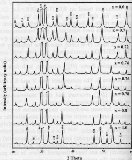
Fig. 2. Powder diffraction pattern of  $\text{Sm}_{1-x}\text{Y}_x\text{TiTaO}_6$  for  $x=0.0, 0.7, 0.72, 0.74, 0.76, 0.78, 0.8$  and  $1.0$ .
