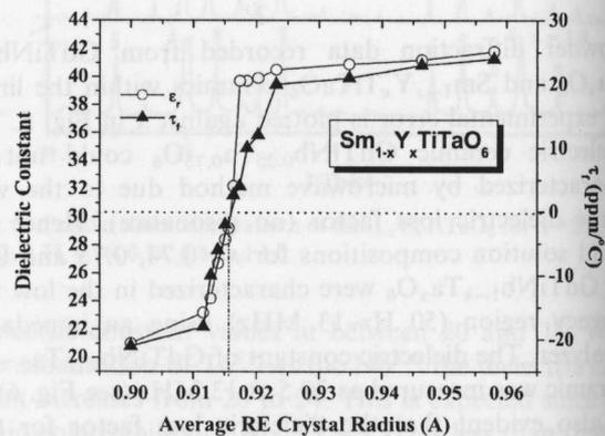
Fig. 11. Variation of  $\tau_r$  and  $\epsilon_r$  with average ionic radius of rare earths in  $\text{Sm}_{1-x}\text{Y}_x\text{TiTaO}_6$ .
