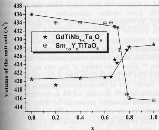
Fig. 5. Variation of unit cell volume of the solid solution phases in GdTiNb<sub>1-x</sub>Ta<sub>x</sub>O<sub>6</sub> and Sm<sub>1-x</sub>Y<sub>x</sub>TiTaO<sub>6</sub> [ $x=0.0–1.0$ ] ceramics.
