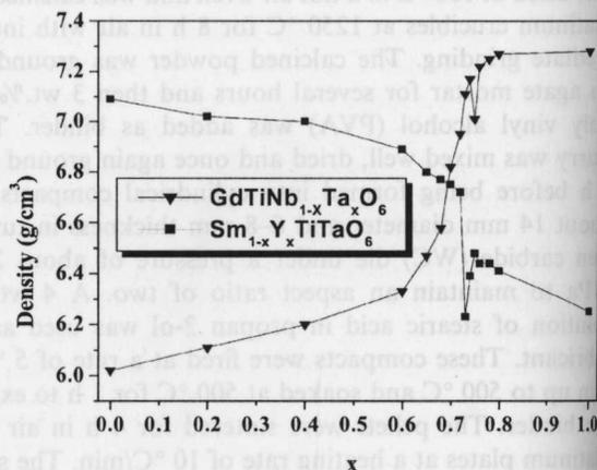
Fig. 3. Variation of bulk density of the solid solution phases with composition  $x$ .
