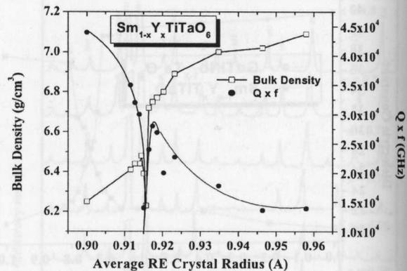
Fig. 10. Variation of bulk density and unloaded quality factor with average ionic radius of rare earths in  $\text{Sm}_{1-x}\text{Y}_x\text{TiTaO}_6$ .
