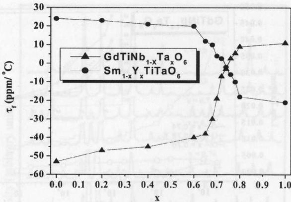
Fig. 8. Variation of the temperature coefficient of resonant frequency  $\tau_r$  with composition  $x$ .
