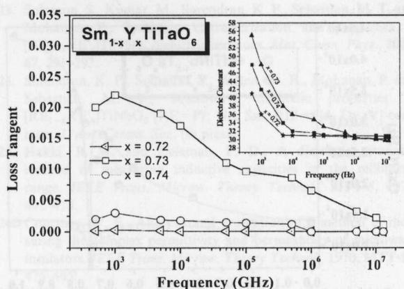
Fig. 7. Variation of the loss tangent and dielectric constant (inset) for  $x=0.72$ ,  $0.73$  and  $0.74$  in Sm<sub>1-x</sub>Y<sub>x</sub>TiTaO<sub>6</sub> in the radio frequency range ( $10^2–1.3 \times 10^7$  Hz).
