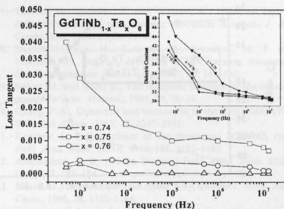
Fig. 6. Variation of the loss tangent and dielectric constant (inset) for  $x=0.74$ ,  $0.75$  and  $0.76$  in GdTiNb<sub>1-x</sub>Ta<sub>x</sub>O<sub>6</sub> in the radio frequency range ( $10^2–1.3 \times 10^7$  Hz).
