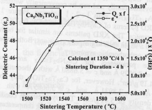
Fig. 3. Variation of dielectric properties of  $\text{Ca}_5\text{Nb}_2\text{TiO}_{12}$  as a function of sintering temperature.
