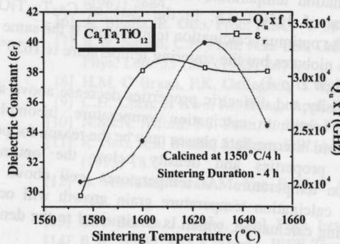
Fig. 4. Variation of dielectric properties of  $\text{Ca}_5\text{Ta}_2\text{TiO}_{12}$  as a function of sintering temperature.
