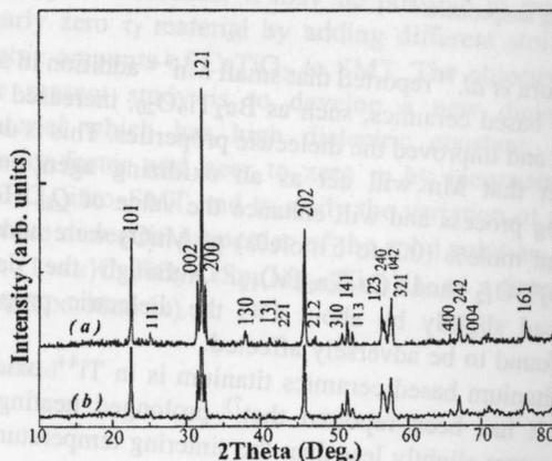
Fig. 1. XRD patterns of (a)  $\text{Ca}_5\text{Nb}_2\text{TiO}_{12}$  and (b)  $\text{Ca}_5\text{Ta}_2\text{TiO}_{12}$  ceramics.
