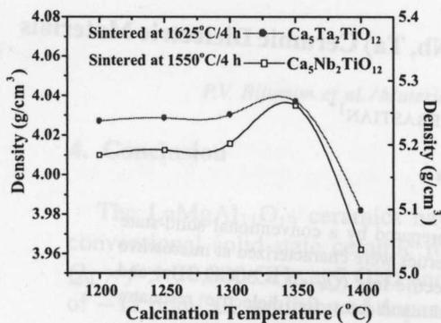
Fig. 2. Variation of density of  $\text{Ca}_5\text{Nb}_2\text{TiO}_{12}$  and  $\text{Ca}_5\text{Ta}_2\text{TiO}_{12}$  ceramics with calcination temperature.
